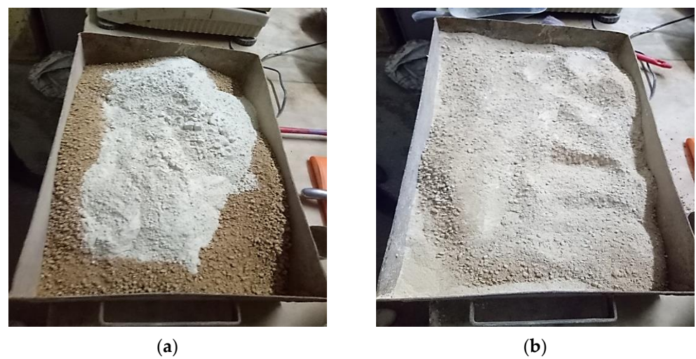
Figure 5. Preparation of soil-bentonite mixture: (a) soil-bentonite, (b) bentonite.
