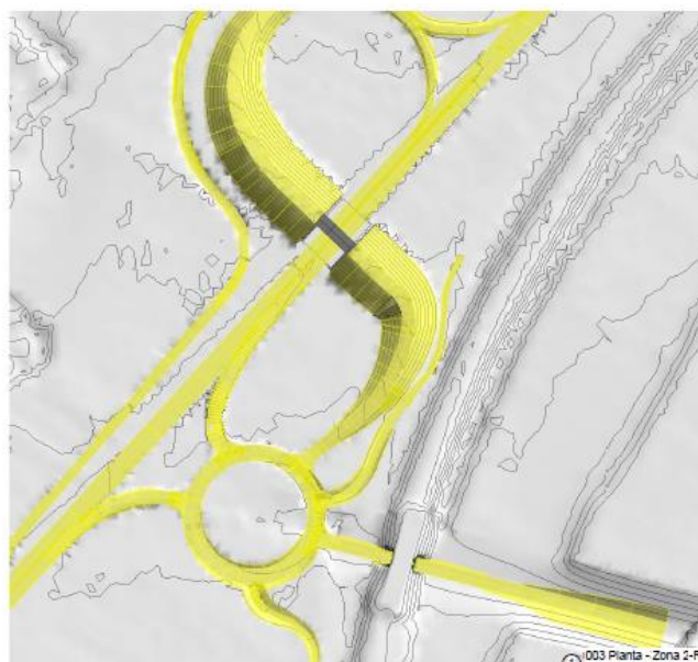
Figure 5. BIM model of the risk of falling to different levels during the execution of the earthworks work unit with the conventional risk assessment.
