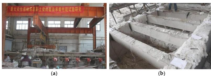
**Figure 2.** Layout of the fire test. (a) The furnace chamber (b) Specimen arrangement in the furnace.
