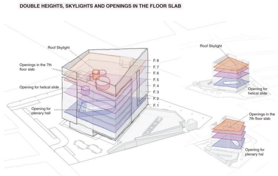
**Figure 14.** Volumetric diagrams of measures taken and actions relating to the following indicators: energy efficiency and green spaces; communications and relationship with the surroundings; shading; double heights, skylights and openings in the floor slab. Source: Created by the author.
