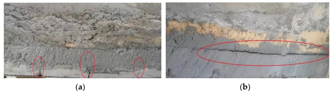
**Figure 7.** Failure phenomena of SP-1 specimen (Failure phenomenon is in the red circle): (a) Local cracking phenomenon; (b) Local debonding phenomenon.
