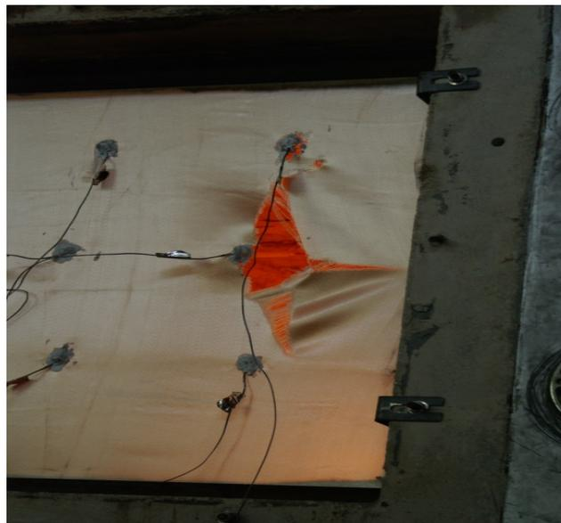
**Figure 8.** The breakdown of the fireproof curtain without a water film.
