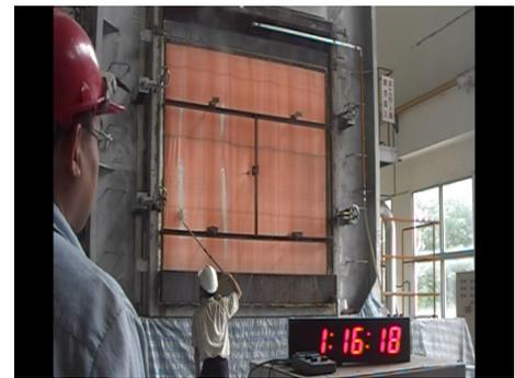
Leakage was measured. The curtain was unburned.
