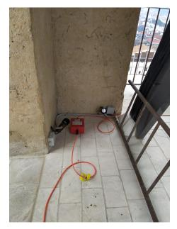
Figure 19. Accelerometer placed on the top of the bell tower, at the height of 22.03 m.
