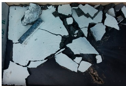
Figure 8. Failure type III. Reprinted/adapted by permission from Springer Nature: Springer Nature Switzerland AG, Mina, A.L.; Trezos, K.G.; Petrou, M.F. Mechanical Properties of Ultra High Performance Fibre Reinforced Concrete and Its Response to Impact Loading. In Advanced Materials for Defense ; Figueiro, R.; Rana, S., Eds.; Springer: Cham, Switzerland, 2020; Volume 4, pp. 71–78.
