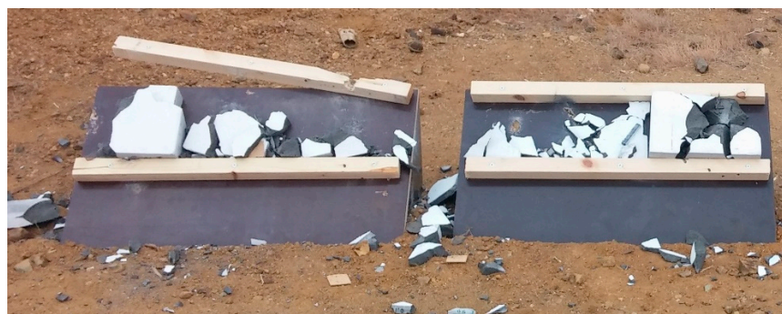
Figure 11. Slabs from mixture 0/16/6 (ultra-high performance concrete, UHPC) and high strength concrete (HSC) after projectile impact test.
