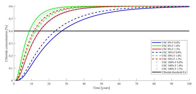
Figure 4. Chloride concentration over time regarding the constant diffusion coefficient.
