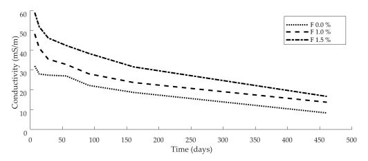
Figure 1. Conductivity of the SLWAC in time with different amounts of fibres.
