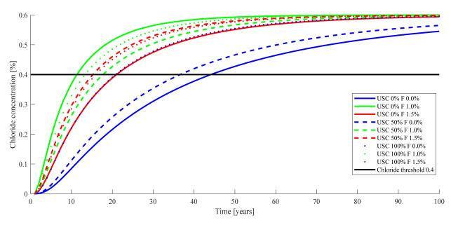
Figure 5. Chloride concentration over time regarding the time-dependent diffusion parameters.
