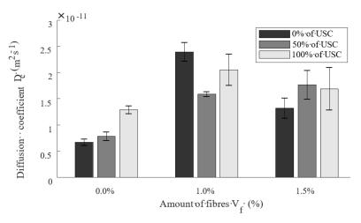
Figure 3. Results of diffusion coefficients at 461 days after concreting for all studied groups.
