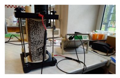
Figure 2. Testing of the bulk resistivity with RCON [14].
