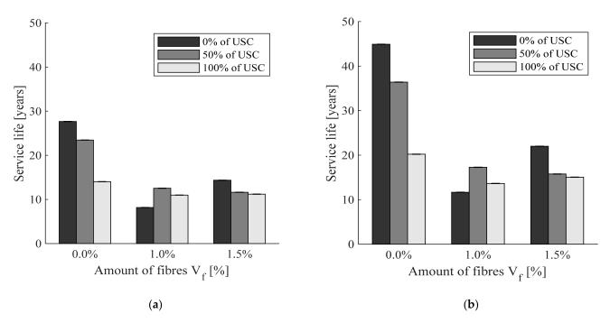
Figure 6. The service life regarding (a) the constant diffusion coefficient and (b) the time-dependent diffusion coefficient.
