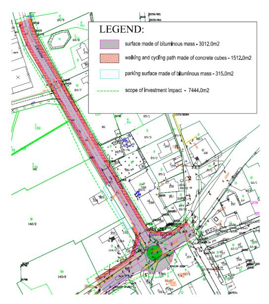
Figure 7. Site plan-proposed solution for the road layout at the intersection—option 2.
