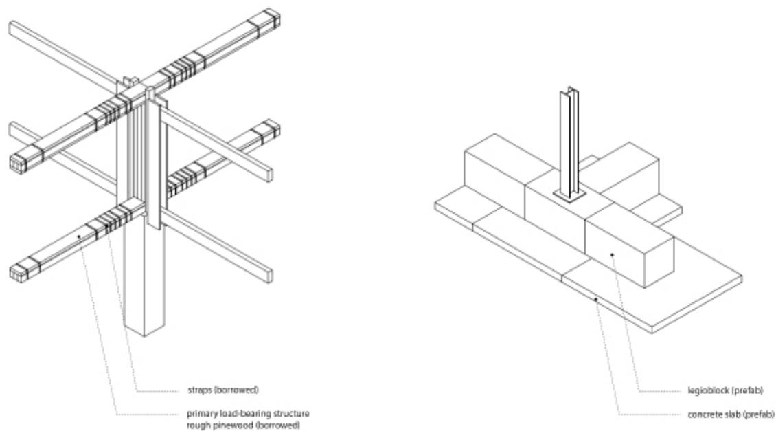
Figure 6. Different building details that were designed for de-/reconstruction.
