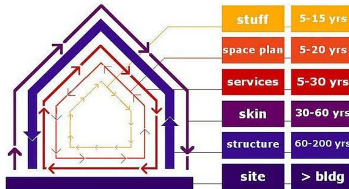
Figure 5. Different layers of the building and their expected time scale [23].
