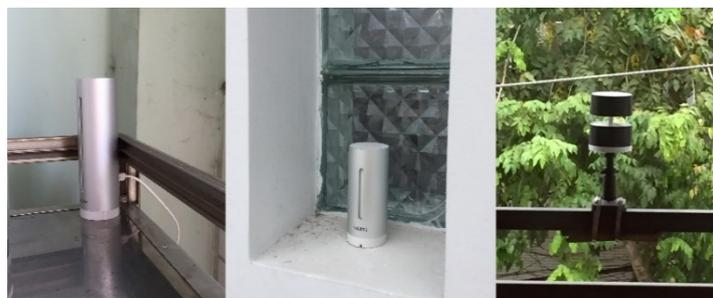
**Figure 5.** Netatmo weather station (outdoor and indoor units, wind gauge).
