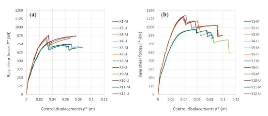
**Figure 11.** Capacity curves determined for the school module 3 (M—modal; U—uniform force pattern): (a) X direction; (b) Y direction.
