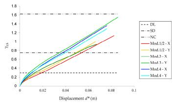
**Figure 17.** Worst-case performance curves determined for each direction of the structural independent modules of the studied "P3" school, and the seismic action levels that are established in the Portuguese National Annex [35] of the EC8-3 for DL, SD and NC limit states.
