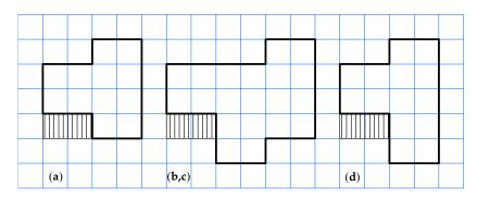
**Figure 2.** Scheme of the classroom modules of the "P3" schools: (a) two classrooms placed in one floor; (b) three classrooms placed in one floor; (c) six classrooms placed in two floors; (d) four classrooms placed in two floors.
