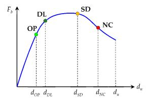
Figure 14. Adopted limit states for damage evaluation.
