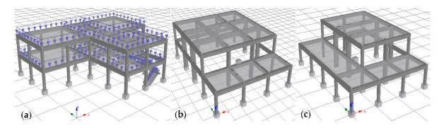
**Figure 8.** SeismoStruct structural models adopted for obtaining the capacity curves: (a) modules 1 and 2; (b) module 3; (c) module 4.
