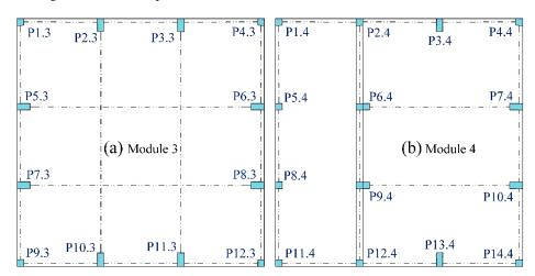
Figure 6. Structural plans of the central modules: (a) module 3; (b) module 4.
