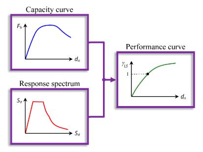
**Figure 16.** Flowchart of the adopted process for obtaining a performance curve for a given capacity curve and response spectrum.
