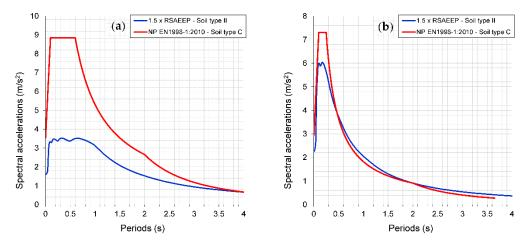
**Figure 13.** Response spectra for the seismic actions that are now established in the Portuguese National Annex of the EC8-1, for school buildings placed in Faro on a ground type C, and the corresponding seismic actions that were established in the national seismic code (RSAEEP) that was mandatory when the studied "P3" school was built: (a) far-field offshore earthquake scenario (type 1); (b) near-source earthquake scenario (type 2).
