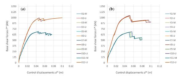
**Figure 12.** Capacity curves determined for the school module 4 (M—modal; U—uniform force pattern): (a) X direction; (b) Y direction.
