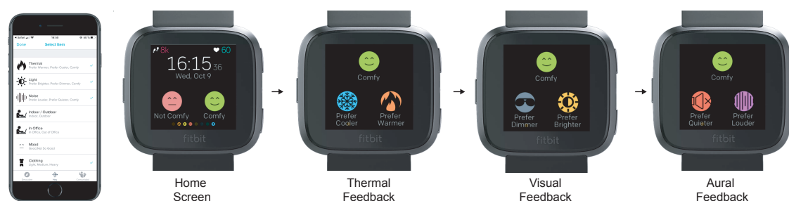
Figure 2. The cozie watch-face, built on the Fitbit smartwatch platform was used to collect subjective feedback. The phone that is paired with the Fitbit can be used to set up additional questions.
