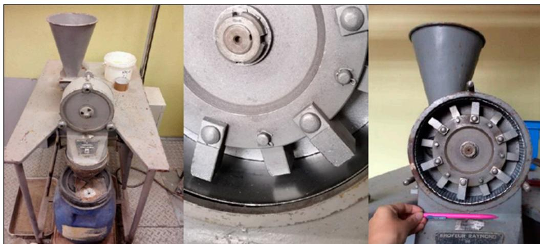
**Figure 1.** Raymond Hammer mill (Laboratoire Stein et Roubaix); **(Left)** the whole equipment; **(Center)** closed-circuit setting (closed lining); and **(Right)** open-circuit setting (dented lining).
