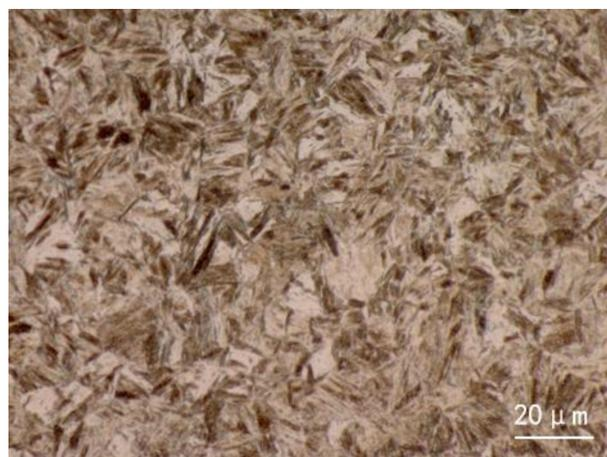
**Figure 1.** Optical microstructure of the hot-stamped hardened steel.
