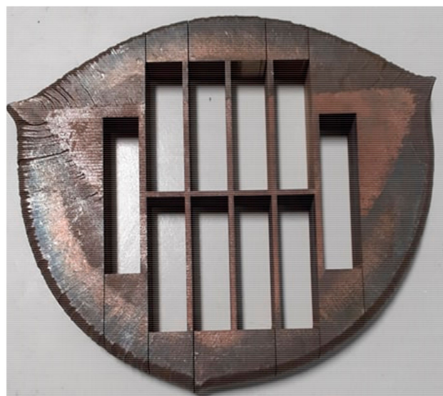
Figure 1. Specimen blank extraction from a pancake forging.
