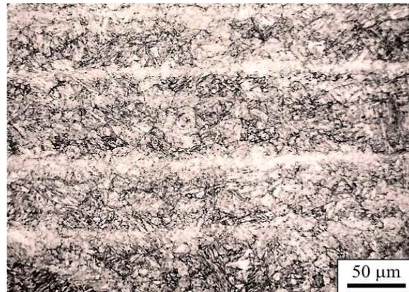
**Figure 5.** Tempered martensite with the remaining shear bands; I TMP; tempering temperature 550 °C.
