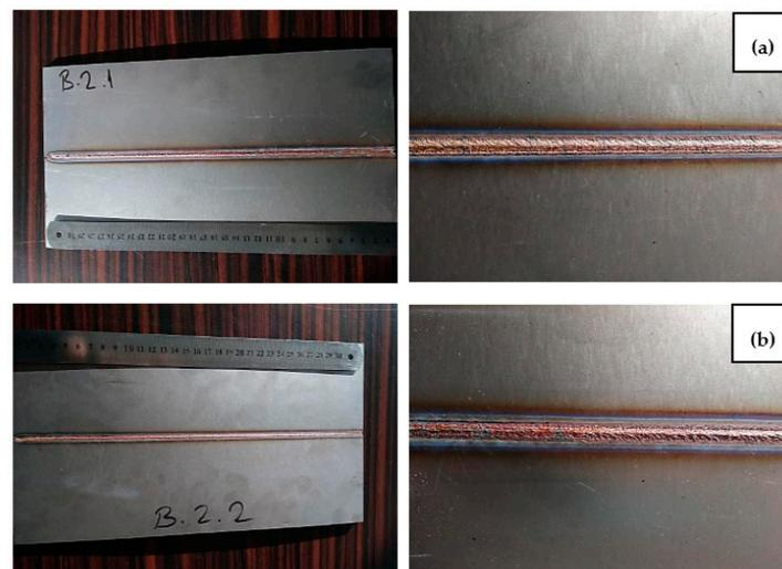
**Figure 2.** Macro images of laser welded joints, (a) A1 Sample, (b) A2 Sample.
