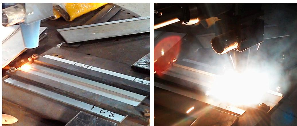
**Figure 1.** The laser welding process and fixing clamps.
