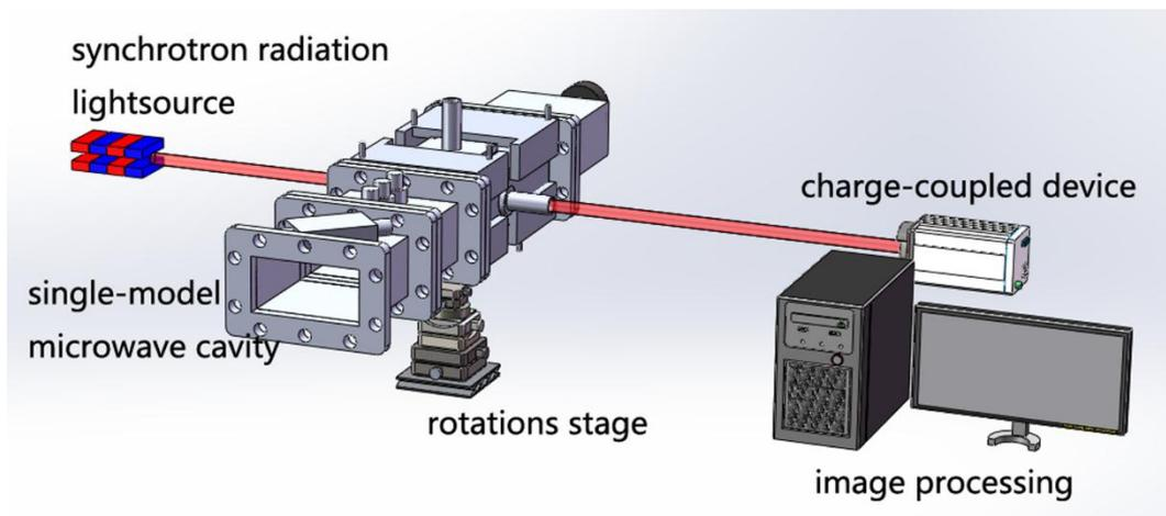
**Figure 1.** Schematic of in situ synchrotron radiation computed tomography (SR-CT) system of microwave sintering.
