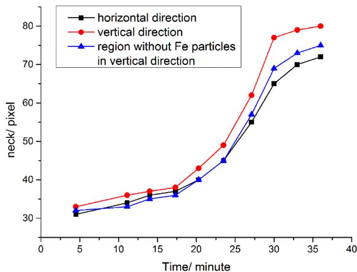
Figure 9. Sintering neck growth curves in different directions in different regions.
