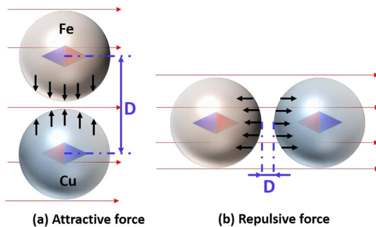
**Figure 4.** Schematic of magnetic force between particles. The magnetic field direction is perpendicular (a) and parallel (b) with the line of two particles' centers.
