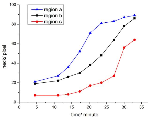
Figure 11. Sintering necks' growth curves of regions with different volume iron particles in the horizontal direction.
