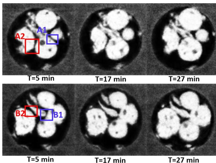
**Figure 12.** Particle shape's influence on sintering neck growth.
