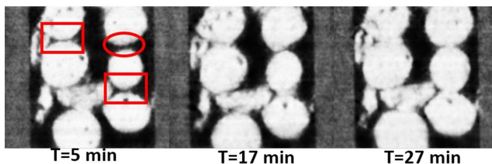
**Figure 7.** Evolution of Cu–Cu necks around iron particles in vertical direction at different sintering times.
