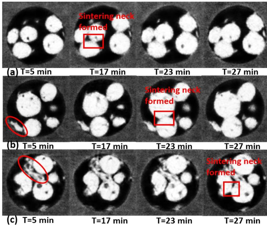
Figure 10. Microstructure evolution of Cu–Cu necks around iron particles in the horizontal direction. (a) no iron particles; (b) a small iron particle; (c) a large iron particle.
