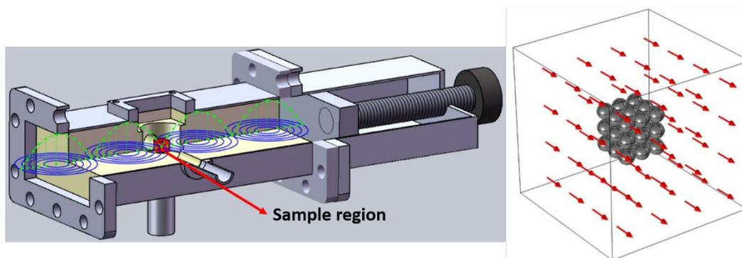
**Figure 5.** Sample position in the microwave magnetic field.
