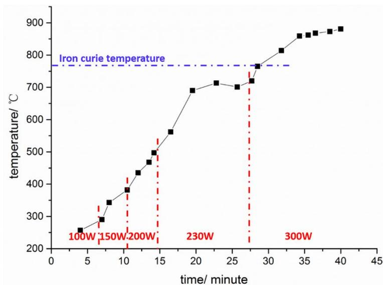
**Figure 2.** Curve of temperature and microwave power.
