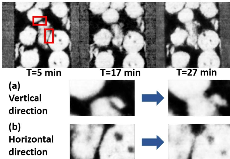
**Figure 6.** Local microstructure evolution of Cu–Fe necks in the vertical direction at different sintering times. Enlarged view of the coupled particles in vertical direction (a) and horizontal direction (b).
