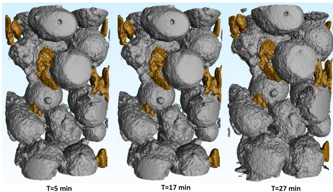
Figure 3. 3D images of the microstructure at different sintering times.
