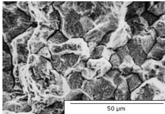
Figure 4. Intergranular brittle fracture of the 316L steel.
