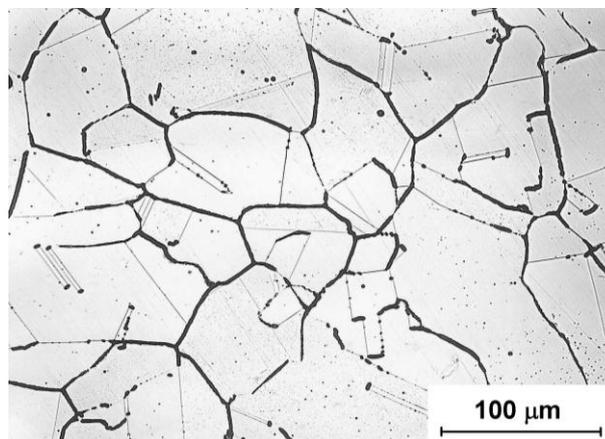
**Figure 3.** Microstructure of 316L steel after solution annealing by regime 1050 °C/1 h/water and sensitization annealing by regime 600 °C/24 h/water.
