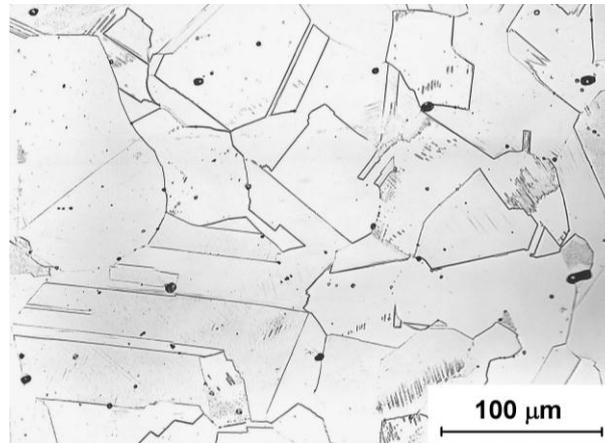
**Figure 1.** Microstructure of the 316L steel after solution annealing by regime 1050 °C/1 h/water.
