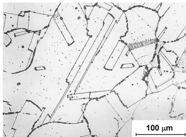
**Figure 2.** Microstructure of the 316L steel after solution annealing by regime 1050 °C/1 h/water and stabilization annealing by regime 850 °C/4 h/water.
