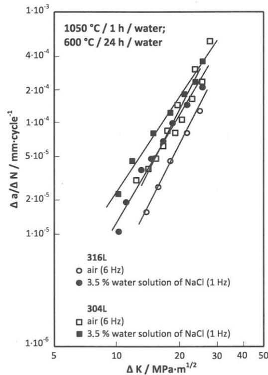
**Figure 7.** Kinetics of fatigue crack growth for 304L and 316L steels after sensitization annealing.
