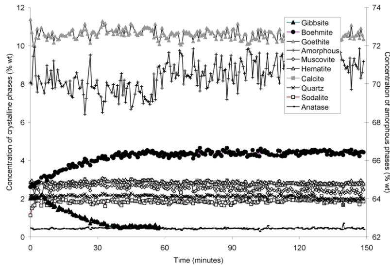
**Figure 5.** Concentration of crystalline and amorphous phases in bauxite residue slurry in capillary reaction vessels as a function of treatment time at 165 °C, as determined by Rietveld-based quantitative mineral analysis of X-ray diffractograms. Note that amorphous content is plotted on the secondary Y axis and represents contributions from X-ray amorphous minerals in bauxite residue, water in the slurry, and the fused silica capillary.
