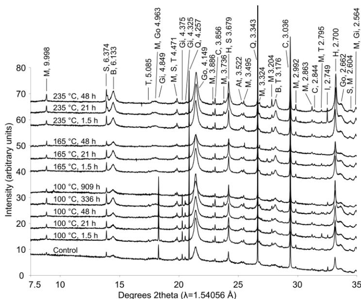
**Figure 7.** X-ray diffraction patterns from bauxite residue before and after hydrothermal treatment. Treatment time and temperature are indicated for each pattern. Peaks between  $7.5^\circ$ – $35^\circ$   $2\theta$  are labeled with d-spacings ( $\text{\AA}$ ) and abbreviations for minerals as follows: M—muscovite; S—sodalite; B—boehmite; T—tricalcium aluminate; Go—goethite; Gi—gibbsite; Q—quartz; C—calcite; H—hematite; At—natase; I—ilmenite.
