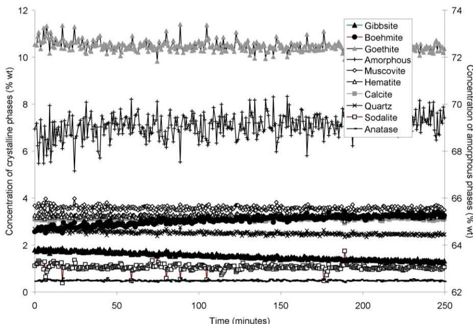
**Figure 3.** Concentration of crystalline and amorphous phases in bauxite residue slurry in capillary reaction vessels as a function of treatment time at 140 °C, as determined by Rietveld-based quantitative mineral analysis of X-ray diffractograms. Note that amorphous content is plotted on the secondary Y axis and represents contributions from X-ray amorphous minerals in bauxite residue, water in the slurry, and the fused silica capillary.
