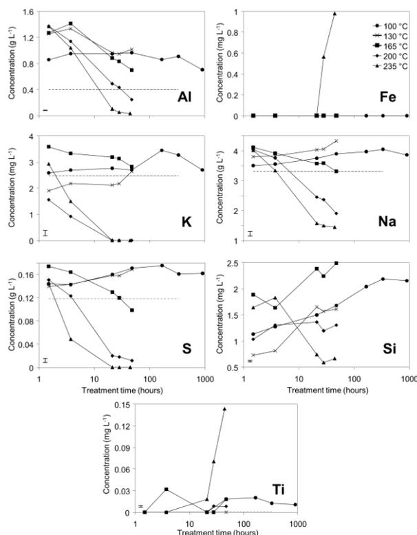
**Figure 2.** Concentrations of selected elements ( $\text{mg}$  or  $\text{g L}^{-1}$ ) in supernatant from bauxite residue after treatment in pressure vessels. Dashed lines indicate concentrations at  $t = 0$ . Where no dashed line is visible, concentrations at  $t = 0$  were below detection limits. Note that treatment time ( $X$  axis) is graphed on a logarithmic scale. Error bars indicate 95% confidence interval for the mean of the 100 °C treatment at 909 h.
