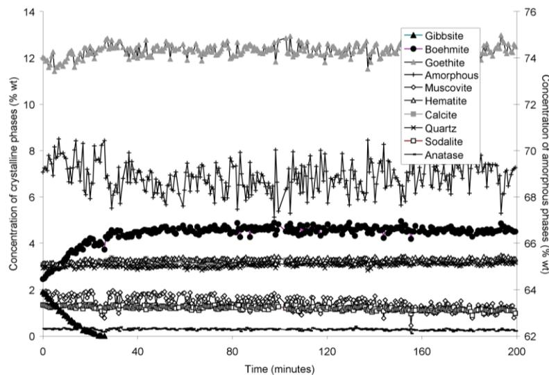
**Figure 6.** Concentration of crystalline and amorphous phases in bauxite residue slurry in capillary reaction vessels as a function of treatment time at 170 °C, as determined by Rietveld-based quantitative mineral analysis of X-ray diffractograms. Note that amorphous content is plotted on the secondary Y axis and represents contributions from X-ray amorphous minerals in bauxite residue, water in the slurry, and the fused silica capillary.
