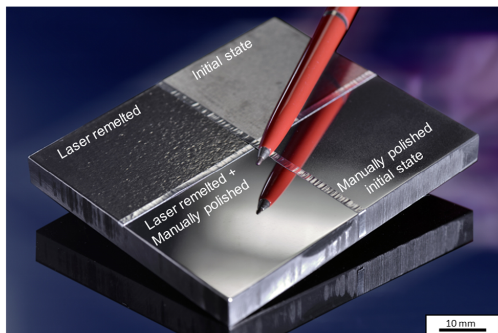
Figure 13. Demonstrator sample after laser remelting and manual polishing.
