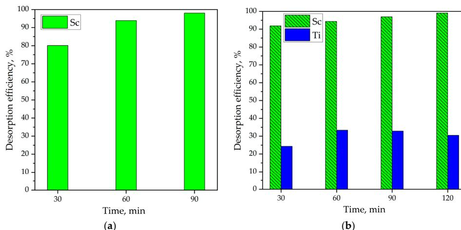
Figure 5. Desorption efficiency with NaHCO<sub>3</sub> solution (200 g L<sup>-1</sup>) from MTS9580, saturated using a model solution (a); PLS (b).
