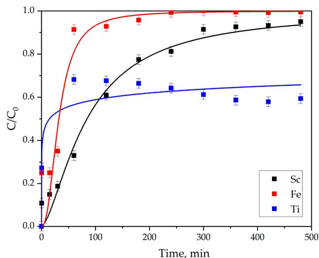
**Figure 4.** MDR model column adsorption on MTS9580 at PLS flow rate of 7.5 mL min<sup>-1</sup>.
