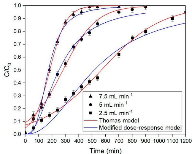
**Figure 3.** Column adsorption of Sc from a simulated solution on MTS9580 at flow rate of 2.5–7.5 mL min<sup>-1</sup>.
