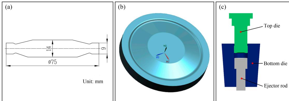
**Figure 1.** Schematic diagram of the formed part and assembly diagram of dies. (a) Two-dimensional drawing of the formed part; (b) three-dimensional model of the formed part; (c) assembly drawing of the forming dies.
