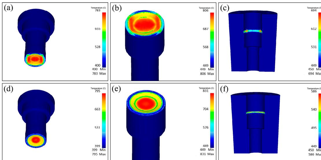
**Figure 8.** Temperature distributions of the dies with (a–c) horizontal billet placement mode and (d–f) vertical billet placement mode. (a,d) Top die; (b,e) ejector rod; (c,f) bottom die.
