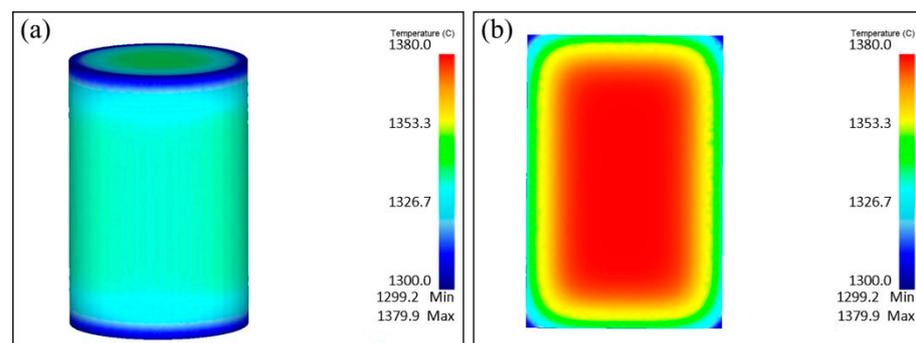
**Figure 4.** Temperature field of the billet after heat transfer to air. (a) The whole billet; (b) the billet section.
