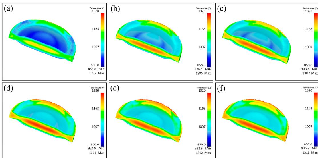
**Figure 10.** Temperature field distribution of the formed parts with different billet temperatures. (a) 1250 °C; (b) 1300 °C; (c) 1350 °C; (d) 1360 °C; (e) 1370 °C; (f) 1380 °C.
