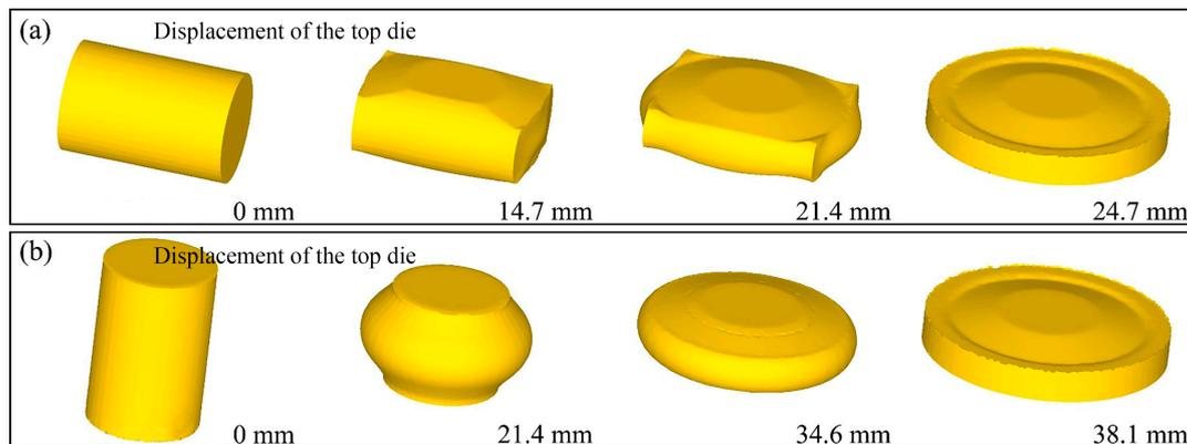
**Figure 6.** The forming process of the billet with different placement modes. (a) Horizontal placement; (b) vertical placement.
