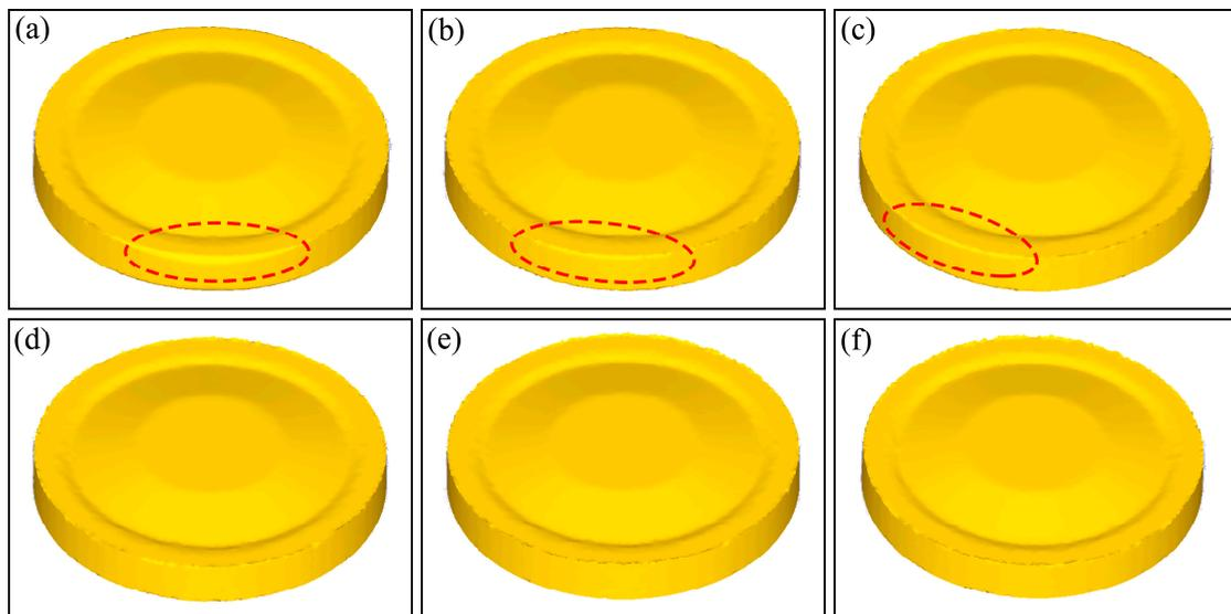
**Figure 9.** Effect of billet temperature on the filling behavior of the formed parts. (a) 1250 °C; (b) 1300 °C; (c) 1350 °C; (d) 1360 °C; (e) 1370 °C; (f) 1380 °C.
