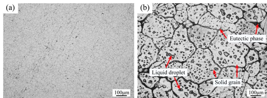
**Figure 3.** Microstructures of the GH4037 alloy. (a) The starting material; (b) the billet heated to 1360  $^{\circ}\text{C}$ .
