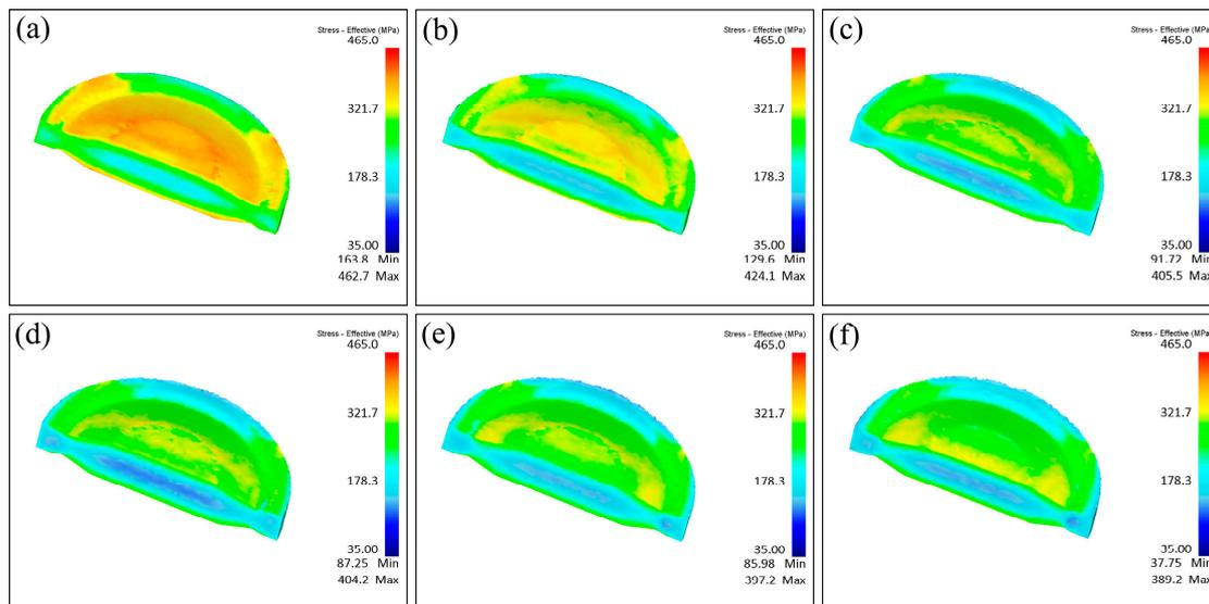
**Figure 11.** Equivalent stress field distribution of the formed parts with different billet temperatures. (a) 1250 °C; (b) 1300 °C; (c) 1350 °C; (d) 1360 °C; (e) 1370 °C; (f) 1380 °C.
