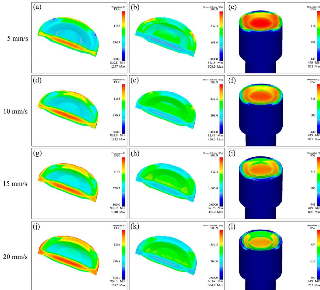
**Figure 12.** (a,d,g,j) The temperature field distribution, (b,e,h,k) equivalent stress field distribution of the formed part, and (c,f,i,l) the temperature field of the ejector rod with different extrusion speeds.
