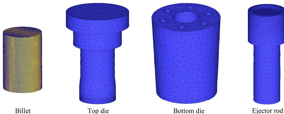
**Figure 2.** Mesh generation models of the billet, top die, bottom die, and ejector rod.
