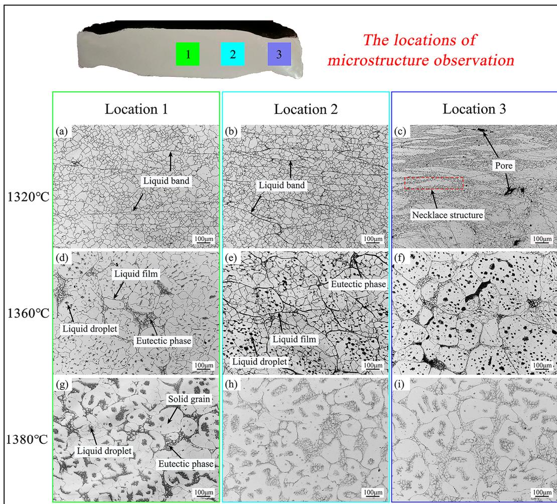
**Figure 14.** Optical microstructures of the formed parts in different locations with different billet temperatures. (a–c) 1320 °C; (d–f) 1360 °C; (g–i) 1380 °C.
