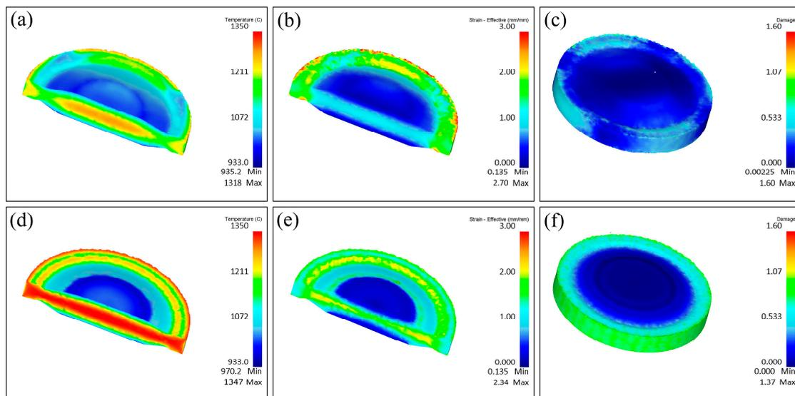
**Figure 7.** Simulation results of the billets with (a–c) horizontal placement mode and (d–f) vertical placement mode. (a,d) Temperature field; (b,e) effective strain field; (c,f) damage field.
