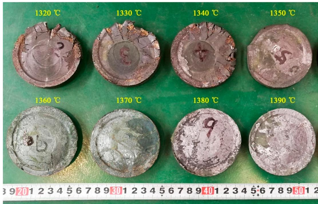
**Figure 13.** Macro morphologies of the formed parts with different billet temperatures.
