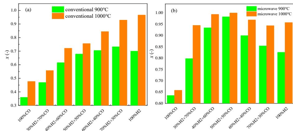
**Figure 8.** Reduction degree of samples during (a) conventional heating at 1000 °C and (b) microwave heating at 1000 °C.
