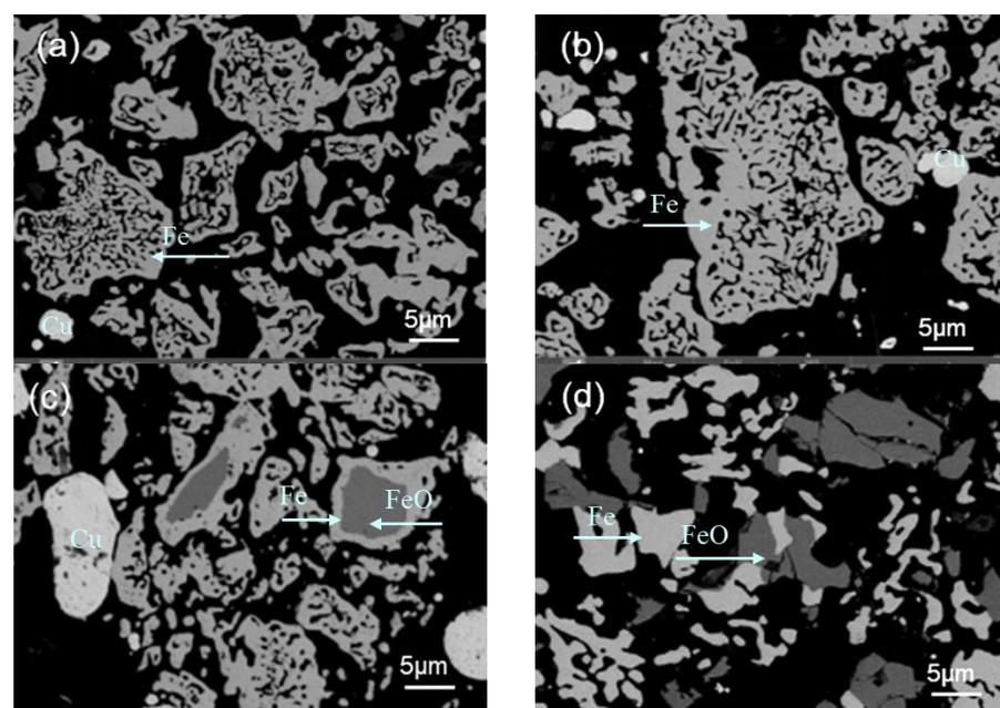
**Figure 9.** Microwave-field-enhanced reduction of magnetite at 1000 °C by (a) 40% H<sub>2</sub> + 60% CO; (b) 60% H<sub>2</sub> + 40% CO; (c) H<sub>2</sub> 100%; (d) CO 100%.
