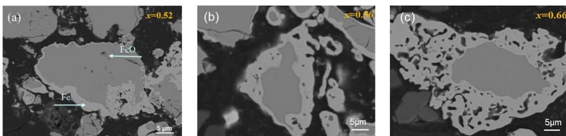
**Figure 5.** Microwave-field-enhanced 30% $\text{H}_2$ -Ar reduction of magnetite at (a) 900 °C; (b) 1000 °C; (c) 1100 °C.
