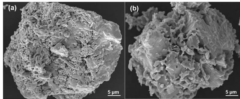
**Figure 7.** Microstructure of magnetite particles: (a) 30% H<sub>2</sub>-Ar; (b) 30% CO-Ar.
