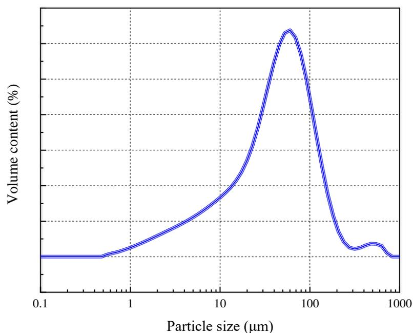
**Figure 2.** Magnetic powder particle distribution map.
