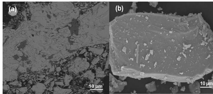
**Figure 4.** Morphology of magnetite particles. (a) SEM image of the cross section of the magnetite particles; (b) SEM image of magnetite particles.
