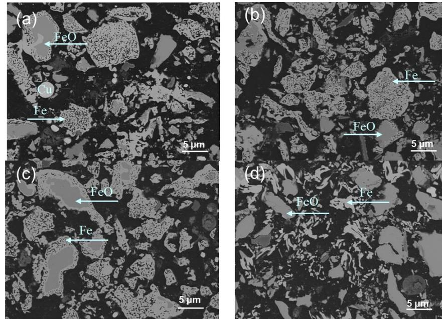
**Figure 10.** Magnetite was reduced under conventional field at 1000 °C by (a) 40% H<sub>2</sub> + 60% CO; (b) 60% H<sub>2</sub> + 40% CO; (c) H<sub>2</sub> 100%; (d) CO 100%.
