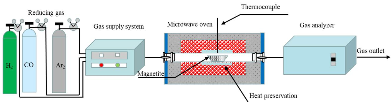
Figure 1. Microwave-heating furnace.
