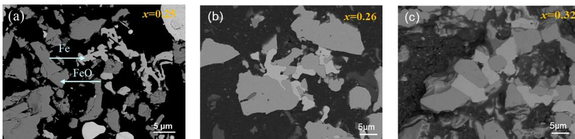
**Figure 6.** Microwave-field-enhanced 30%CO-Ar reduction of magnetite at (a) 900 °C; (b) 1000 °C; (c) 1100 °C.
