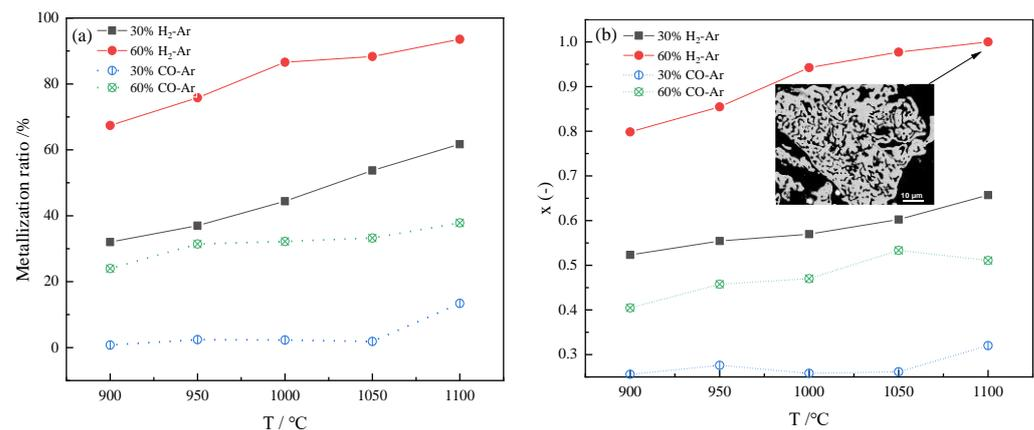
**Figure 3.** H<sub>2</sub> and CO reduction of magnetite under microwave field: (a) metallization ratio (b) reduction degree.
