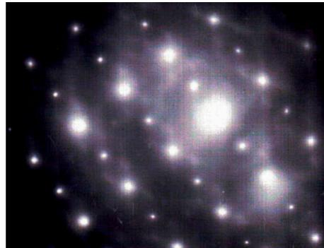
**Figure 2.** Microdiffraction pattern of the  $[\bar{1}17]$ -oriented  $\text{Ti}_{49.7}\text{-Ni}_{50.3}$  (at.%) alloy single crystals after hydrogenation, showing only reflexes of the B2 phase. Zone axis  $(110)_{\text{B2}}$ .
