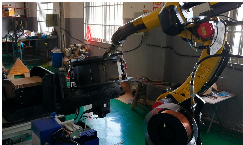
Figure 23. Experimental scenario for impeller welding.
