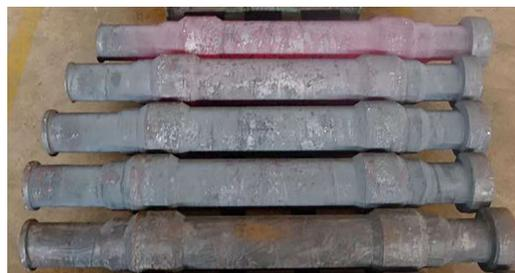
**Figure 20.** Some railway axles obtained by CWR experiment.
