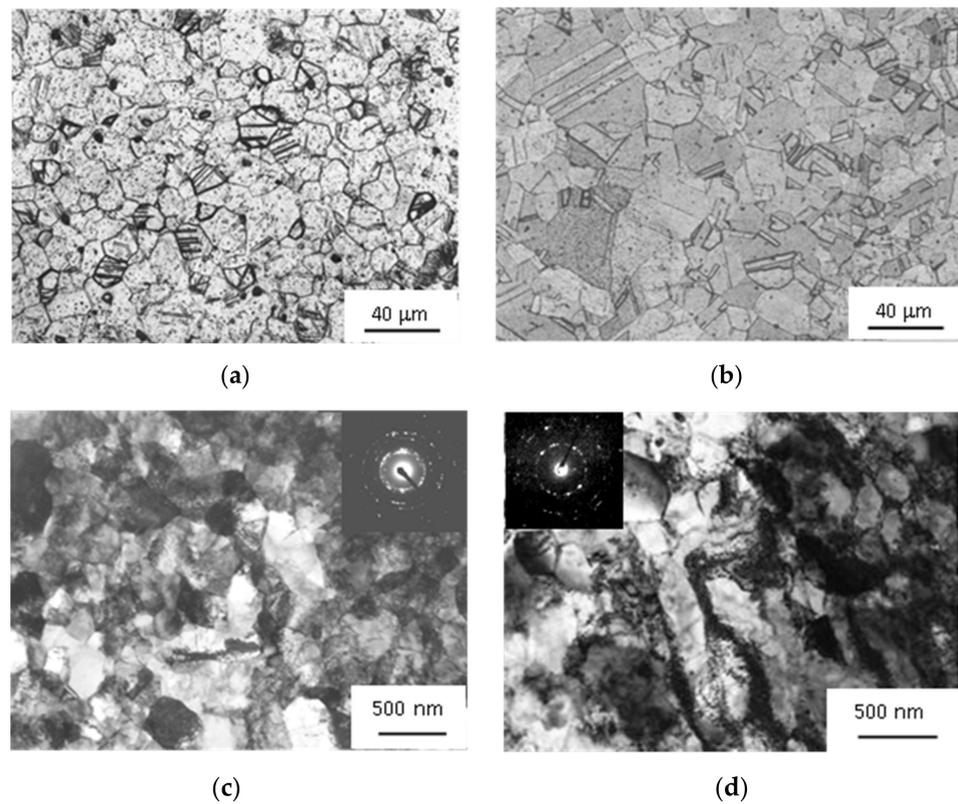
**Figure 2.** Microstructure and microdiffraction images in cross section for titanium (a,c) and copper (b,d) in states: (a,b)—as-received (optical); (c,d)—ultrafine-grained (TEM).
