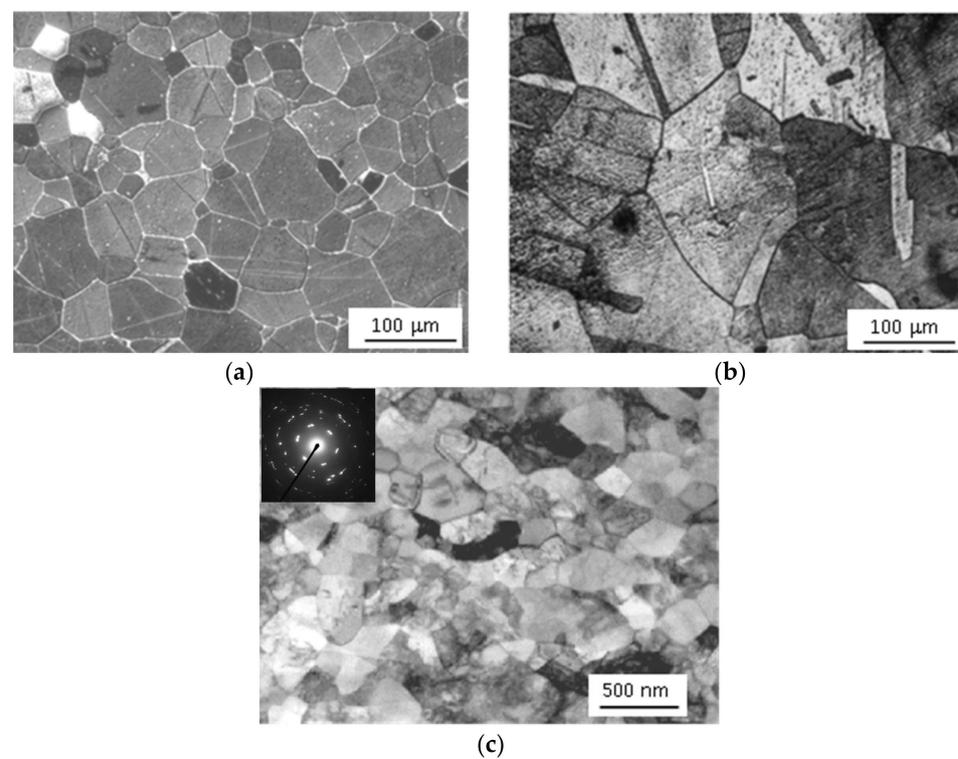
**Figure 3.** Microstructure images in cross section for ECAP titanium (a,c) and ECAP copper (b) in states: (a,b)—after annealing at 600 °C (optical); (c)—after annealing at 300 °C (TEM).
