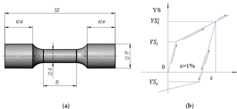
**Figure 1.** Sample view and dimensions for tension–compression (a) and loading scheme (b).
