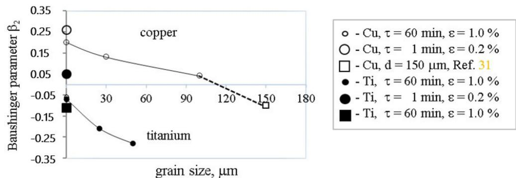
**Figure 5.** Grain size dependence of Bauschinger parameter  $\beta_2$  in copper and titanium, data from [31].
