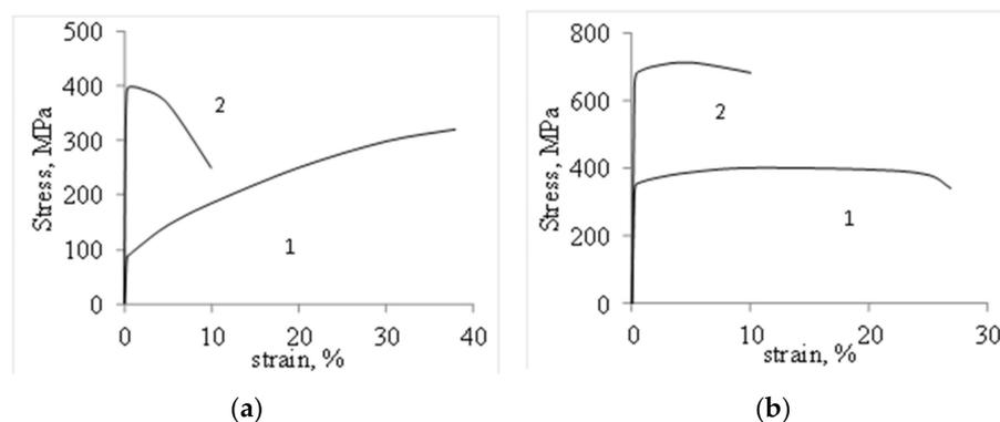
**Figure 4.** Typical stress–strain curves for copper (a) and titanium (b) in as-received state (curve 1) and ultrafine-grained state (curve 2).
