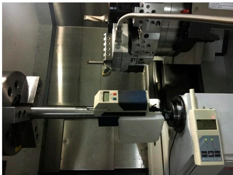
**Figure 1.** Measuring setup of surface roughness tester and cutting sound.
