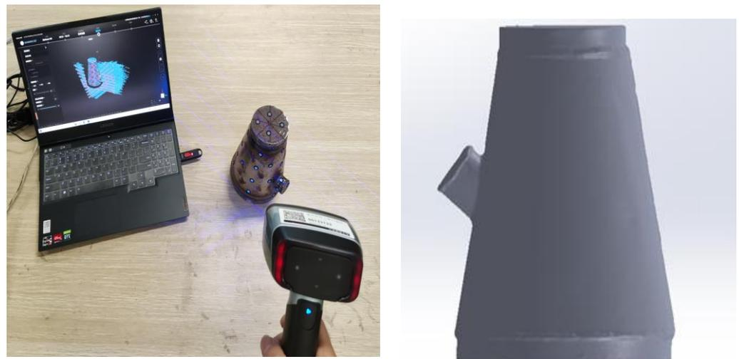
**Figure 6.** Three-dimensional scanning.
