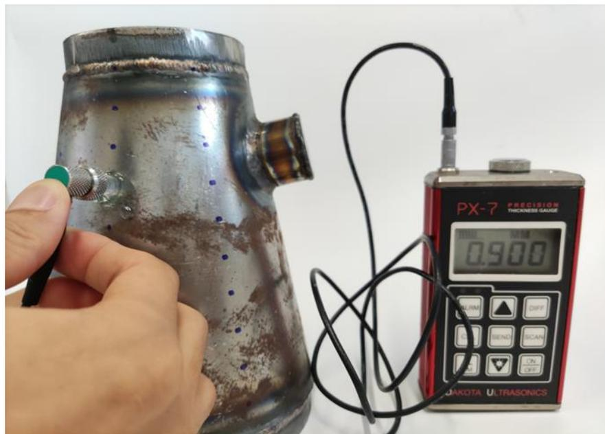
Figure 4. Sample model actual thickness measurement.
