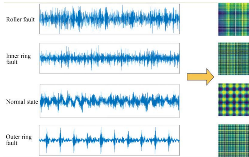
Figure 7. Time-domain waveforms and GAF diagrams.
