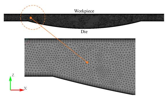
Figure 8. Computational mesh of fluid domain with micro-pocket textured surface.
