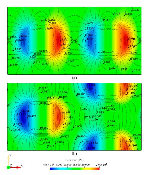
Figure 23. Velocity (line contours) and pressure (coloured contours) distributions at the mid-plane between the die and workpiece: (a) grid array pattern; (b) crossing array pattern. Note that the unit of velocity is mm/s.
