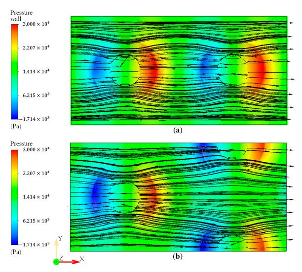
**Figure 24.** Streamlines and pressure (coloured contours) distributions around the die surface: (a) grid array pattern; (b) crossing array pattern.
