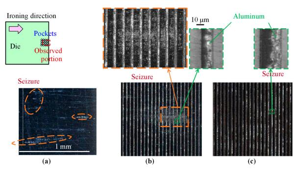
**Figure 14.** Occurrence of seizure on die with (**a**) smooth surface at r = 15% and with grooved array pattern,  $h = 2 \mu m$ ,  $L = 50 \mu m$ , groove width d of (**b**) 15  $\mu$ m at r = 7%, and (**c**) 30  $\mu$ m at r = 6%.
