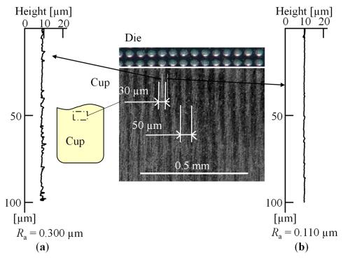
**Figure 17.** The die surface before ironing and the cup surface obtained after ironing with a grid array pattern having  $d = 30 \mu m$ ,  $h = 2 \mu m$ , and  $L = 50 \mu m$ , applying a lubricant containing extreme pressure additive at r = 17%; surface roughness and 2D profiles (**a**) on pocket marks, and (**b**) outside pocket marks.
