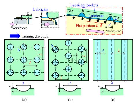
**Figure 1.** Schematic illustration of array patterns of micro-lubricant pockets: (a) grid, (b) crossing, and (c) grooved array patterns.
