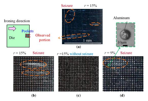
**Figure 10.** Occurrence of seizure on die with (**a**) smooth surface at r = 15% and with grid array pattern,  $d = 30 \, \mu m$ ,  $L = 50 \, \mu m$ , pocket depth h of (**b**) 1  $\mu m$  at r = 15%, (**c**) 2  $\mu m$  at r = 15%, and (**d**) 6  $\mu m$  at r = 9%.
