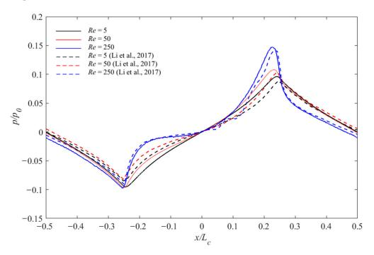
**Figure 6.** Static pressure distribution on the middle section of the micro-pocket unit at different Reynolds numbers [38].
