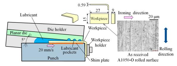
Figure 3. Strip ironing of aluminum alloy sheets illustrated in half-section view (scale in mm).
