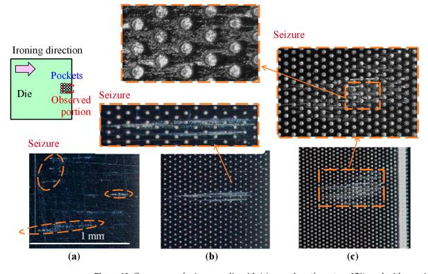
**Figure 13.** Occurrence of seizure on die with (**a**) smooth surface at r = 15%, and with crossing array pattern,  $h = 2 \mu m$ ,  $L = 50 \mu m$ , pocket diameter d of (**b**) 15  $\mu m$  at r = 15%, and (**c**) d of 30  $\mu m$  at r = 12%.
