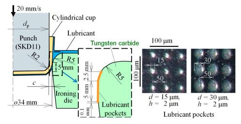
Figure 4. Ironing conditions for SUS430 stainless steel cylindrical cups and die surfaces.
