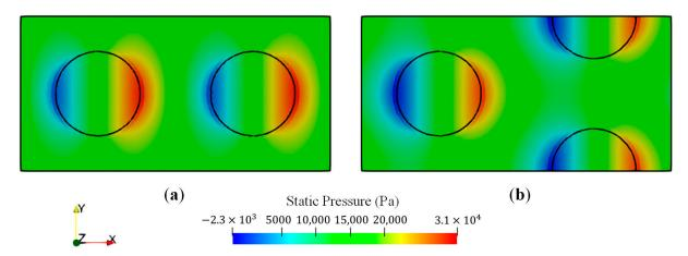
**Figure 21.** Static pressure distribution on the die surface: (a) grid array pattern; (b) crossing array pattern. The circle shows where the pockets are approximately located.
