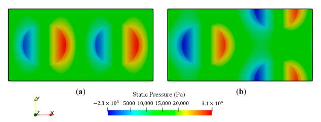
**Figure 22.** Static pressure distribution on the workpiece surface: (a) grid array pattern; (b) crossing array pattern.
