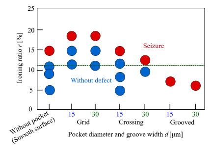
**Figure 15.** Ironing limit of die having lubricant pockets with different array patterns,  $h = 2 \mu m$  and  $L = 50 \mu m$ .
