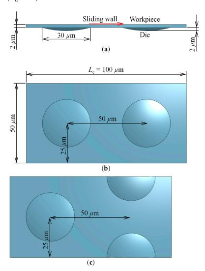
**Figure 5.** Geometrical model of the simplified contacting couple and the computational fluid domain with micro-lubricant pockets: (a) side view; (b) top view (grid array pattern); (c) top view (crossing array pattern).
