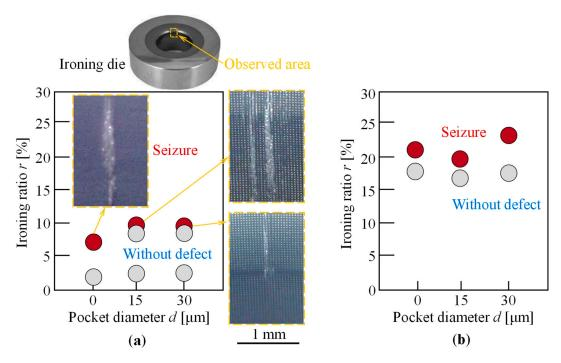
**Figure 18.** Ironing limit of laser textured dies having lubricant pockets used to iron SUS430 stainless steel cups by applying lubricant (a) without an extreme pressure additive, and (b) with an extreme pressure additive.
