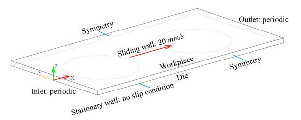
**Figure 7.** Fluid domain and boundary conditions of a two parallel contacting couple between the die and the workpiece with thin-film lubrication.
