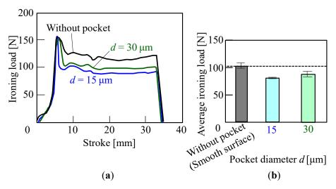
**Figure 12.** Ironing load of aluminum alloy sheets with grid array patterns,  $h = 2 \mu m$ ,  $L = 50 \mu m$  and r = 10%: (a) load-travel diagram and (b) average ironing load.
