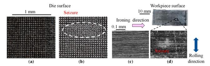
**Figure 9.** Optical micrograph of the die and workpiece surfaces after ironing with grid array pattern,  $d = 30 \, \mu m$ ,  $h = 2 \, \mu m$  and  $L = 50 \, \mu m$ : (a) die surface without seizure at r = 15%; (b) seizure on die surface at r = 18%; (c) workpiece surface without seizure at r = 15%; and (d) seizure on workpiece surface at r = 18%.
