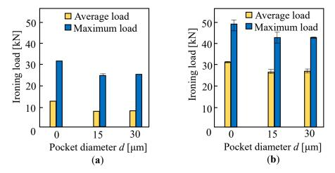
**Figure 19.** Ironing load of laser textured dies having lubricant pockets used to iron SUS430 stainless steel cups by applying lubricant (**a**) without an extreme pressure additive at r = 3%, and (**b**) with an extreme pressure additive at r = 8%.
