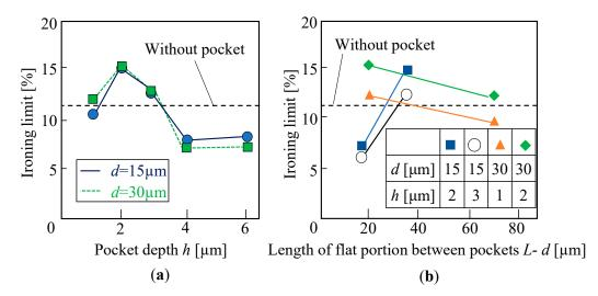
**Figure 11.** Effect of (a) pocket depth at  $L = 50 \mu m$  and (b) length of flat portion between pockets on the ironing limit with grid array pattern.
