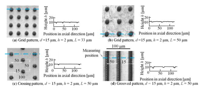
**Figure 2.** Micrographs and 2D profiles of array patterns of micro-lubricant pockets: grid array pattern having  $d = 15 \mu m$ ,  $h = 2 \mu m$  (a)  $L = 33 \mu m$  and (b)  $L = 50 \mu m$ ; (c) crossing array pattern having  $d = 15 \mu m$ ,  $h = 2 \mu m$ ,  $L = 50 \mu m$ ; (d) grooved array pattern having  $d = 15 \mu m$ ,  $h = 2 \mu m$ ,  $L = 50 \mu m$ .
