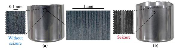
**Figure 16.** Stainless steel cup obtained after ironing with a grid array pattern having  $d = 30 \mu m$ ,  $h = 2 \mu m$ , and  $L = 50 \mu m$ , applying lubricant containing an extreme pressure additive at (**a**) r = 17%, and (**b**) at r = 23%.
