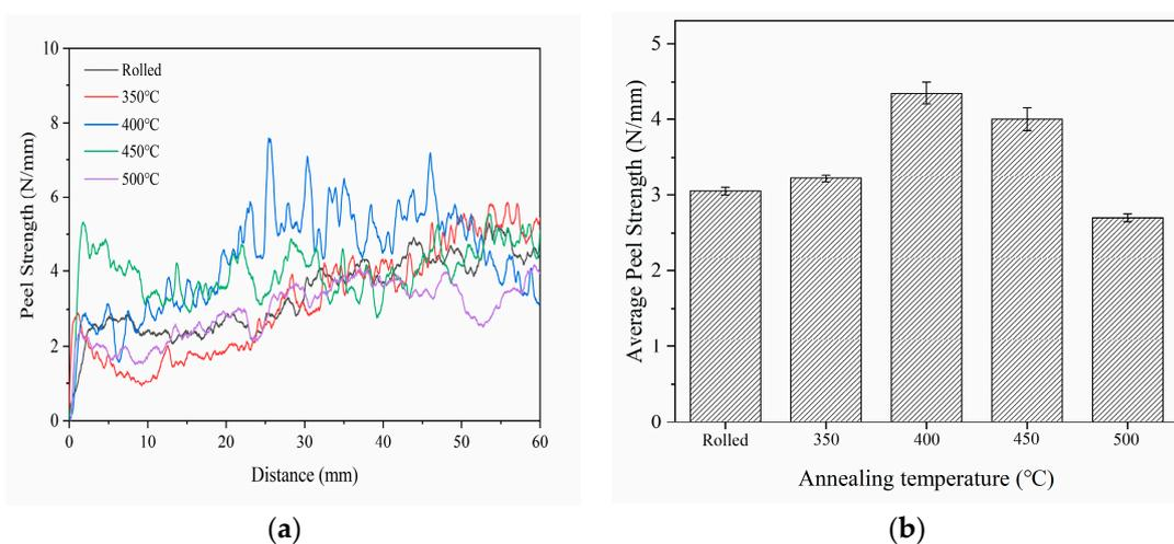
**Figure 9.** Variation curve of ultra-thin Cu/Al composite sheets' peel force at different annealing temperatures. (a) Peel strength value; (b) Average peel strength value.
