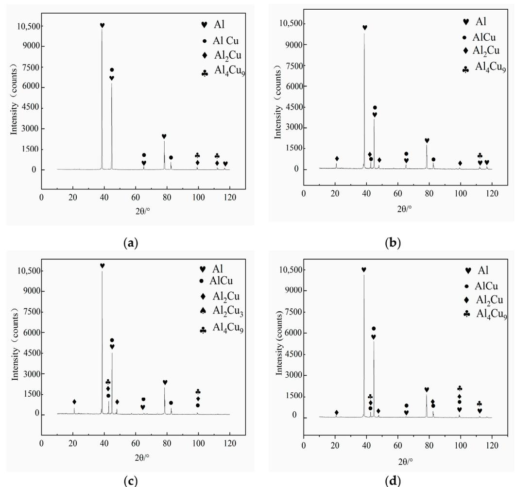
**Figure 10.** The X-ray diffraction patterns at the interface diffusion layer of ultra-thin Cu/Al composite sheets at four annealing temperatures: (a) 350 °C; (b) 400 °C; (c) 450 °C; (d) 500 °C.
