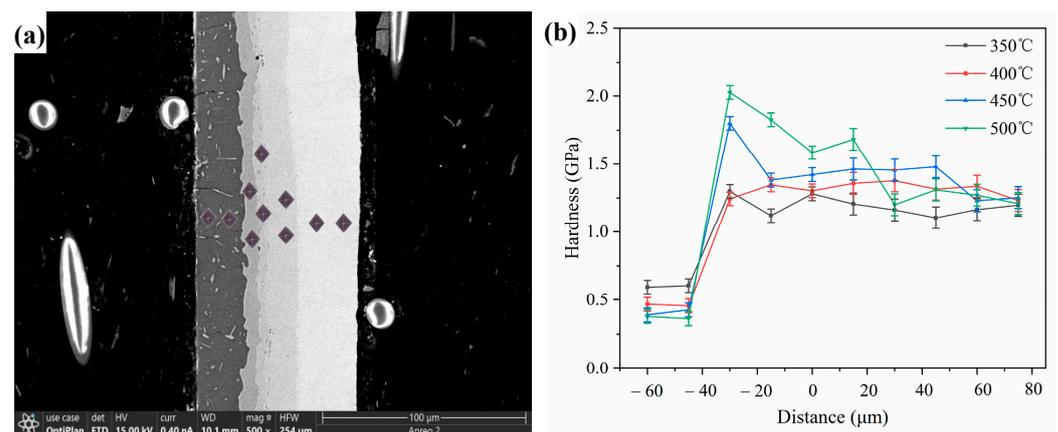
**Figure 5.** Variation curve of microhardness on both sides of the interface of ultra-thin Cu/Al composite sheets at different annealing temperatures. (a) Dotting position; (b) Hardness value.
