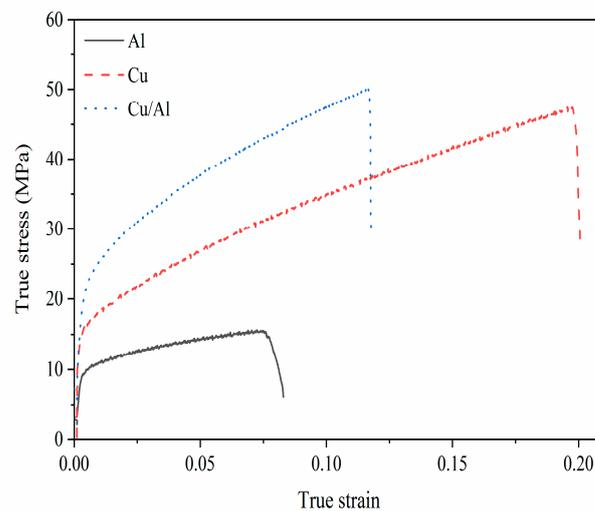
**Figure 6.** True stress–true strain curves of pure Cu, pure Al and ultra-thin Cu/Al composite sheets at the same annealing temperatures.
