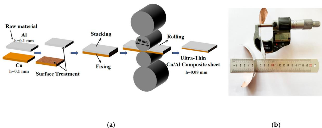
**Figure 1.** (a) Rolling process of ultra-thin Cu/Al composite sheet. (b) Rolling products.
