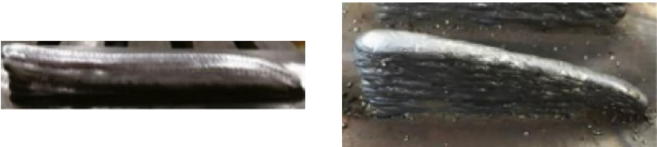
**Figure 9.** Uneven bead height, adapted from [17].
