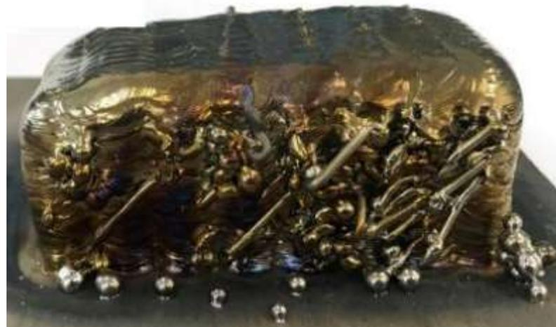
**Figure 7.** Unmelted wire in WAAM, adapted from [18].
