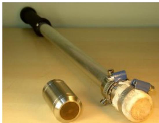
**Figure 12.** EMAT transducer on the left as it is, and on the right with heat protection, adapted from [31].
