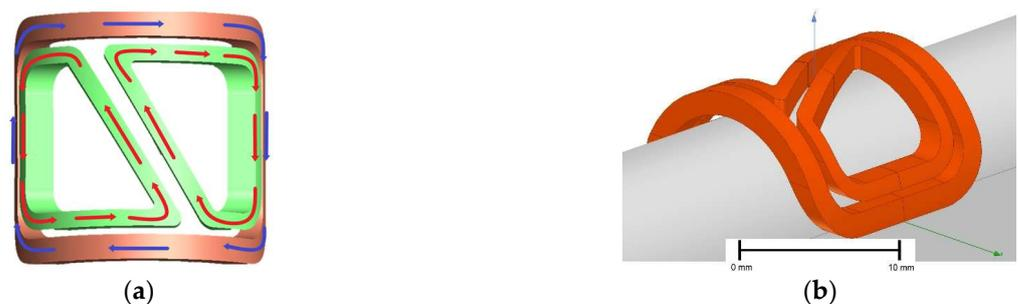
**Figure 19.** Concept probe with the best performance simulated. (a) Top view of the probe with the excitation coil represented in red and the sensing coils in green; (b) Probe modeled in Ansys Electronics used for the simulations.
