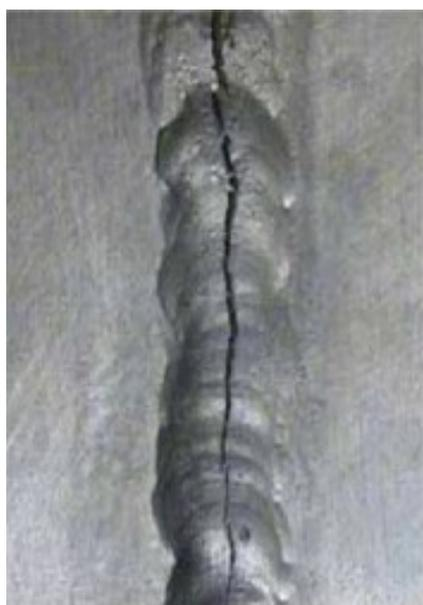
**Figure 3.** Weld crack adapted from [12].
