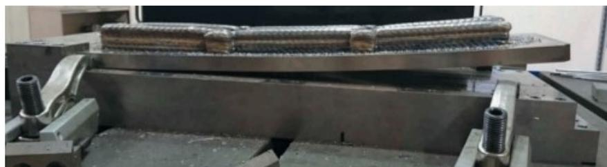
**Figure 10.** Geometric distortion, adapted from [24].
