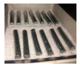
Figure 5. Sintered tensile test blanks.
