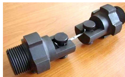
Figure 5. Specimen fixing assembly.
