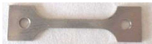
Figure 4. Small-sized flat tensile specimen.
