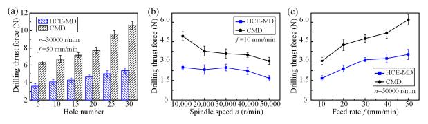
**Figure 11.** Drilling thrust force of the HCE-MD and CMD. (**a**) Change with hole number; (**b**) change with spindle speed; (**c**) change with feed rate.
