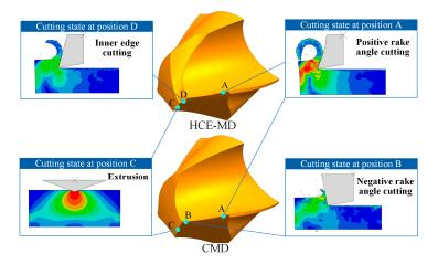
Figure 2. Cutting state of micro-drill cutting edge.
