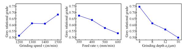
Figure 9. Influence of process parameters on the grey relational grade.
