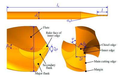
Figure 1. Schematic diagram of the HCE-MD geometric structure.
