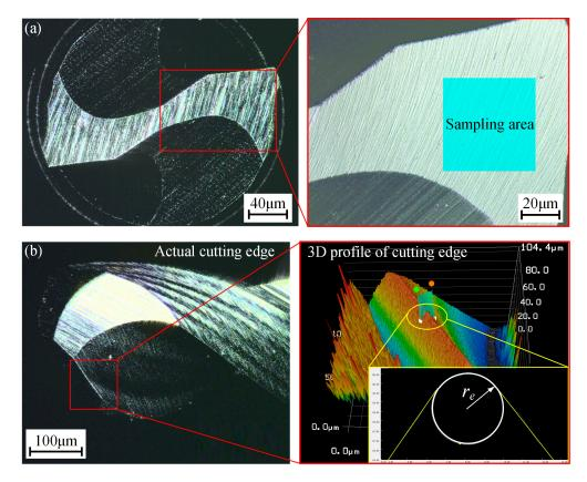
**Figure 4.** (**a**) Measurement method of the flank roughness; (**b**) measurement method of the micro-drill edge radius.
