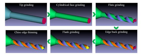
Figure 5. Grinding process of the HCE-MD.
