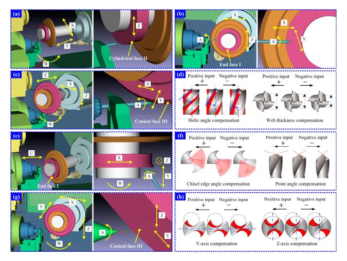
**Figure 6.** Schematic diagram of machining principle for each process. (**a**) Tip grinding; (**b**) cylindrical face grinding; (**c**) flute grinding; (**d**) micro compensation of flute characteristic parameters; (**e**) flank grinding; (**f**) micro compensation of flank characteristic parameters; (**g**) CE thinning; (**h**) micro compensation of the thinned CE dimension.
