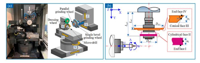
**Figure 3.** Tool grinding experimental device. (**a**) Structure of tool grinding machine; (**b**) structure and position of grinding wheel.
