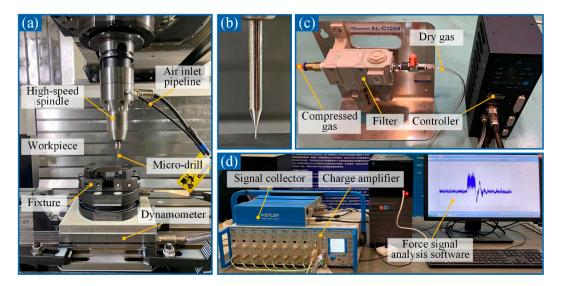
**Figure 7.** Micro-drilling experimental device. (**a**) Experimental process; (**b**) micro-drill; (**c**) supporting components for high-speed spindle; (**d**) supporting components for dynamometer.
