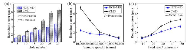
**Figure 14.** Micro-hole roundness error of the HCE-MD and CMD. (**a**) Change with hole number; (**b**) change with spindle speed; (**c**) change with feed rate.
