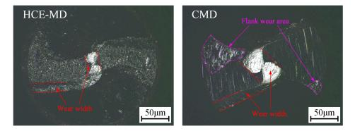
Figure 12. Wear morphology of drill tip.
