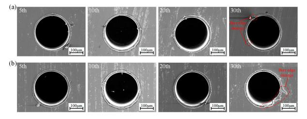
**Figure 13.** Micro-hole entrance morphology. (**a**) Micro-holes produced by HCE-MD; (**b**) micro-holes produced by CMD.
