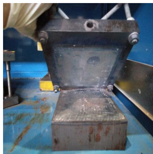
Figure 2. Heated blocks used for bainitic quench.
