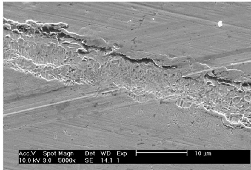
**Figure 6.** Crevice corrosion detected in a groove on a retrieved archwire (used for at least 6 months) caused by orthodontic pliers (reproduced by permission of Oxford University Press on behalf of the European Orthodontic Society, from [106]).
