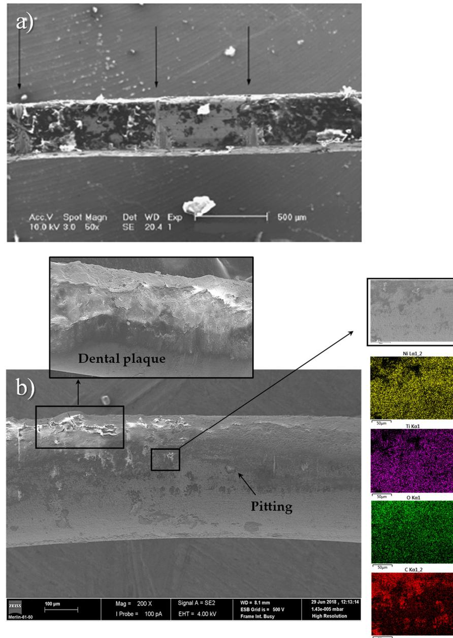
**Figure 9.** SEM micrographs of retrieved archwires: (a) SS archwires before cleaning, showing plaque and food remnants on the surface and evident marks of the location of the bracket borders (black arrows) (reproduced by permission of Oxford University Press on behalf of the European Orthodontic Society, from [106]); (b) SEM micrographs and EDS elemental distribution maps of an NiTi archwire after 17 weeks of intraoral use (reproduced from [116]).
