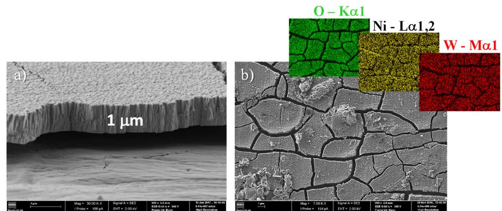
**Figure 18.** SEM micrographs of as-deposited W–N sputtered coatings (a) and its surface morphology after (b) Fusayama–Meyer solution aging (37 °C, 30 days, pH 8.3) coupled with EDS elemental maps distribution (adapted from [468], own work).
