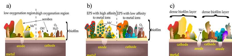
**Figure 8.** MIC mechanisms on a metallic surface in the oral cavity: (a) cells with varying degrees of oxygenation; (b) cells with different concentration of metal ions; and (c) passive–active cells. EPS: extracellular polymeric substances (reproduced from [73]).
