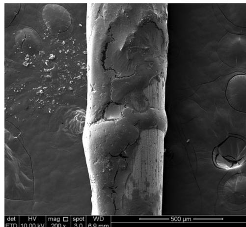
**Figure 20.** Epoxy coating loss on an archwire when exposed to acidic artificial saliva (reprinted from [474], Copyright (2020), with permission from Elsevier).
