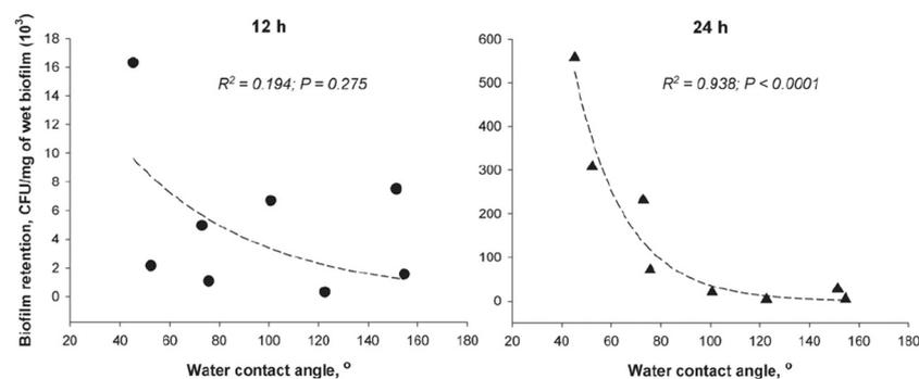
**Figure 21.** Biofilm retention after 12 and 24 h of incubation as a function of the water contact angle on organosilane coated brackets (used with permission of IOP Publishing, Ltd., from [509]; permission conveyed through Copyright Clearance Center, Inc.).
