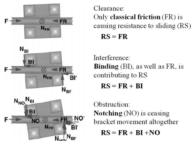
**Figure 11.** Schematic representations of the resistance to sliding components in a bracket/archwire contact (reproduced by permission of Oxford University Press on behalf of the European Orthodontic Society, from [218]).
