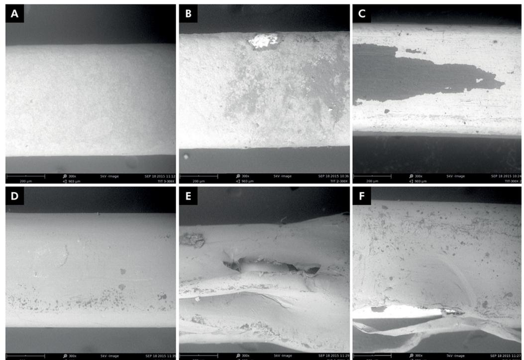
**Figure 19.** Photomicrographs of coated wires: (A) as-received Titanol® Cosmetic, (B,C) post clinical Titanol® Cosmetic, (D) as-received Biocosmetic, (E,F) post clinical Biocosmetic (reproduced from [488]).
