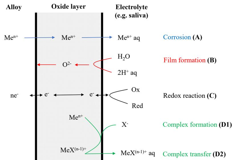
**Figure 5.** Passivation model of a metallic surface in an electrolyte. Me: metal element; X: complexing anions, e.g.,  $\text{Cl}^-$  and  $\text{F}^-$ . (used with permission of John Wiley & Sons—Books, from [97]; permission conveyed through Copyright Clearance Center, Inc.).
