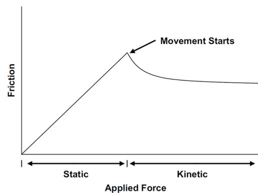
**Figure 12.** The two types of friction present when a force is applied to an object. Static friction occurs until a certain limit above which the movement starts. Kinetic friction opposes the on-going movement (reprinted from [215], Copyright (2009), with permission from Elsevier).
