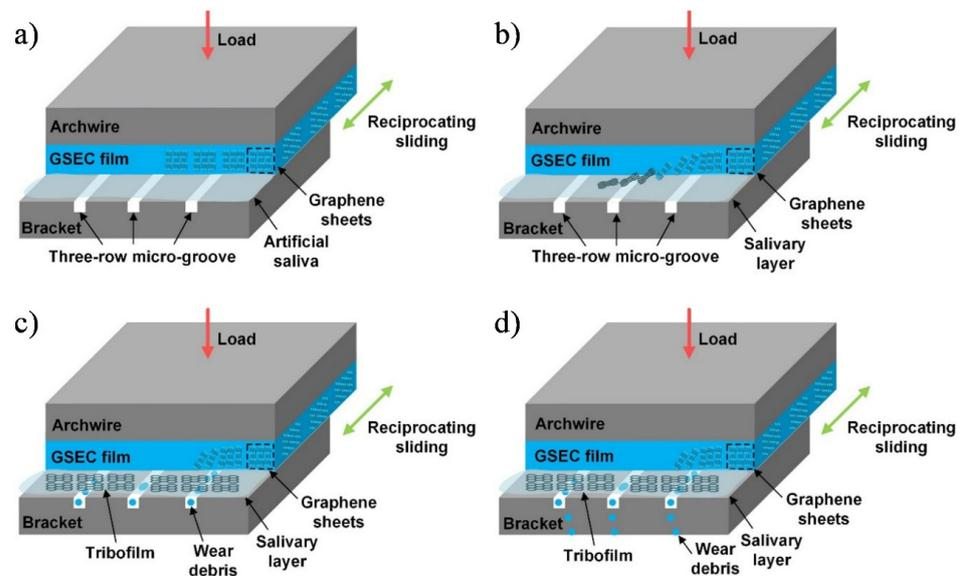
**Figure 23.** Low friction mechanism of graphene sheets embedded carbon (GSEC) coating on an SS archwire against an SS bracket: (a) initial state of the contact combination; (b) stable low friction with the formation of graphete-rich tribofilm and salivary adsorbed layer; (c) accumulation of wear debris detached from the GSEC film with micro-groove; and (d) flow out of wear debris with artificial saliva from the micro-groove (reproduced from [556]).
