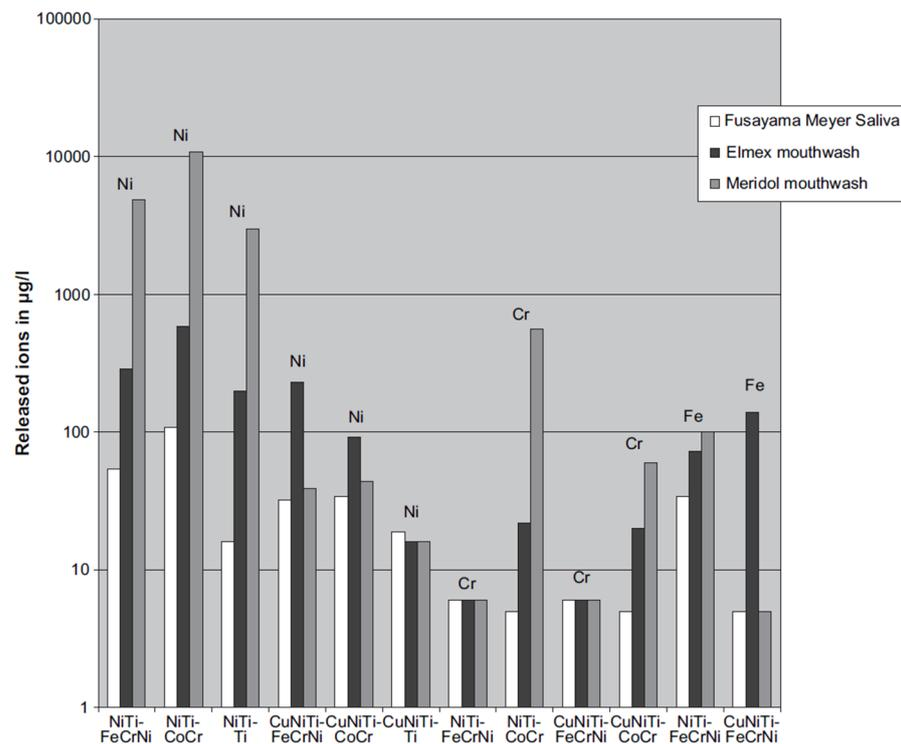
**Figure 14.** Metal ions (in µg/L) released by wire-bracket combinations in three different solutions (reprinted by permission of Oxford University Press on behalf of the European Orthodontic Society, from [108]; permission conveyed through Copyright Clearance Center, Inc.).
