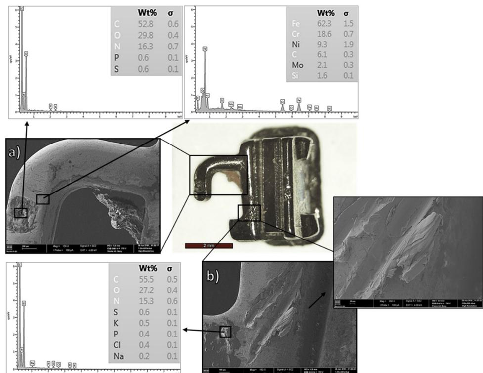
**Figure 13.** Optical and SEM micrographs of a retrieved SS tube after 2 years of intraoral exposure: (a) cavity filled with organic material; (b) wear track and debris coupled with the EDS chemical composition (reproduced from [116]).
