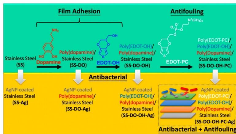
**Figure 22.** A complex polymeric-based composite deposited onto an SS flat substrate to confer the surface with antibacterial and antifouling properties (reprinted with permission from [518]. Copyright (2020) American Chemical Society).
