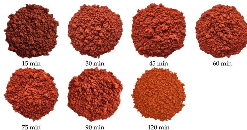
**Figure 5.** Images of the spent  $\text{LiFePO}_4$  cathode materials at different roasting times.
