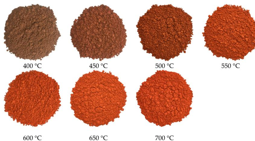
**Figure 3.** Images of the spent  $\text{LiFePO}_4$  cathode materials at different roasting temperatures.
