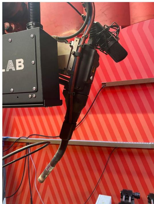
**Figure 1.** Attachment of microphone to welding arm.
