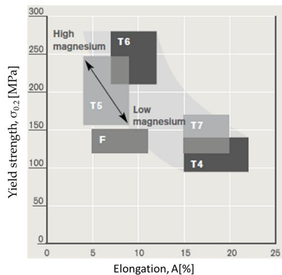
**Figure 3.** Impact of heat treatment processes on the elongation and strength of HPDC alloys [15].
