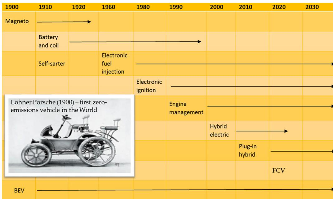
Figure 1. The historical perspective of road vehicle electrification [5].
