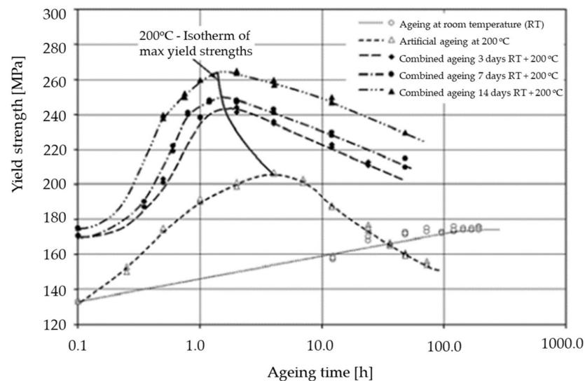
**Figure 4.** Increases in the yield strength through a combination of natural and artificial ageing at 200 °C; the isotherm shows the influence of natural ageing time on the maximum strength [16].
