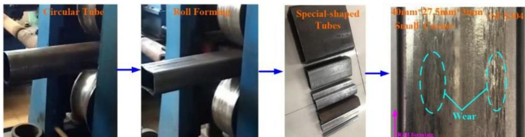
**Figure 7.** Roll forming test.
