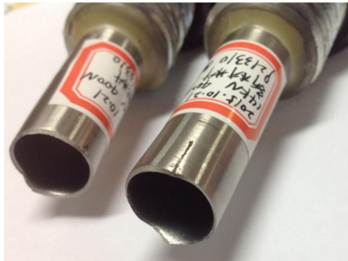
Figure 3. Fracture morphology of the fretting fatigue tube specimen.
