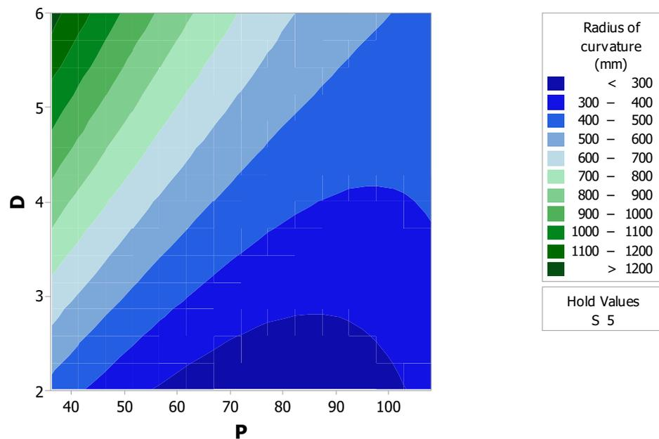
Figure 4. The interaction between laser power and distance between irradiation lines on the radius of curvature.
