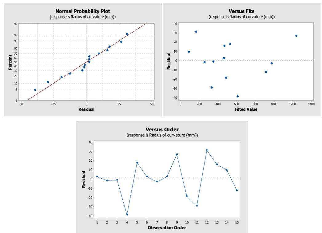
**Figure 2.** Normal probability plots for radius of curvature.
