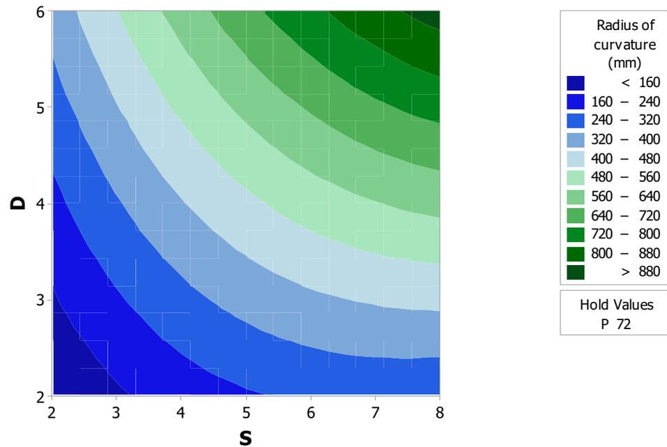
**Figure 5.** The interaction between scanning speed and distance between irradiation lines on the radius of curvature.
