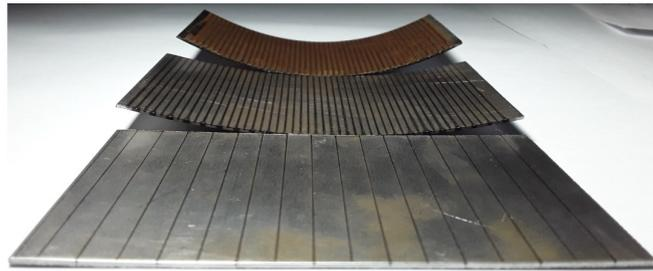
**Figure 1.** Some of the laser-formed cylindrical surfaces from primary sheets with dimensions of 1 mm (thickness)  $\times$  100 mm (length)  $\times$  60 mm (width), obtained from different input parameters.
