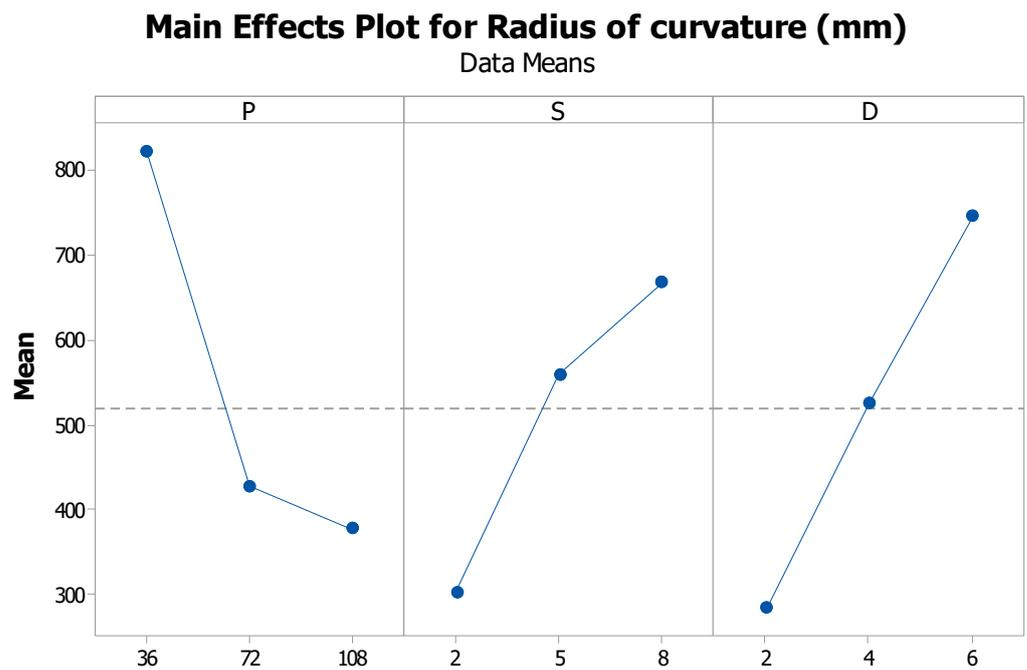
Figure 3. The effects of input parameters on the radius of curvature of laser-formed cylindrical surfaces.
