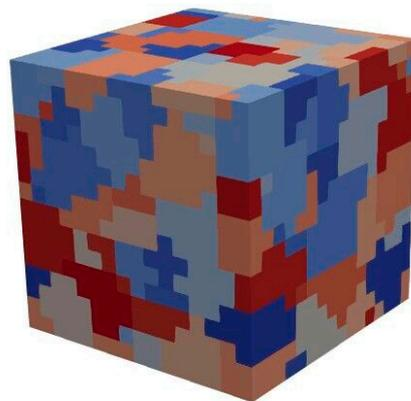
**Figure 6.** The representative volume element (RVE) used for simulation.
