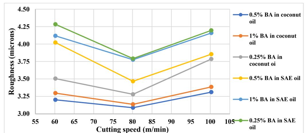
Figure 7. The variation of the surface roughness with the cutting speed [67].
