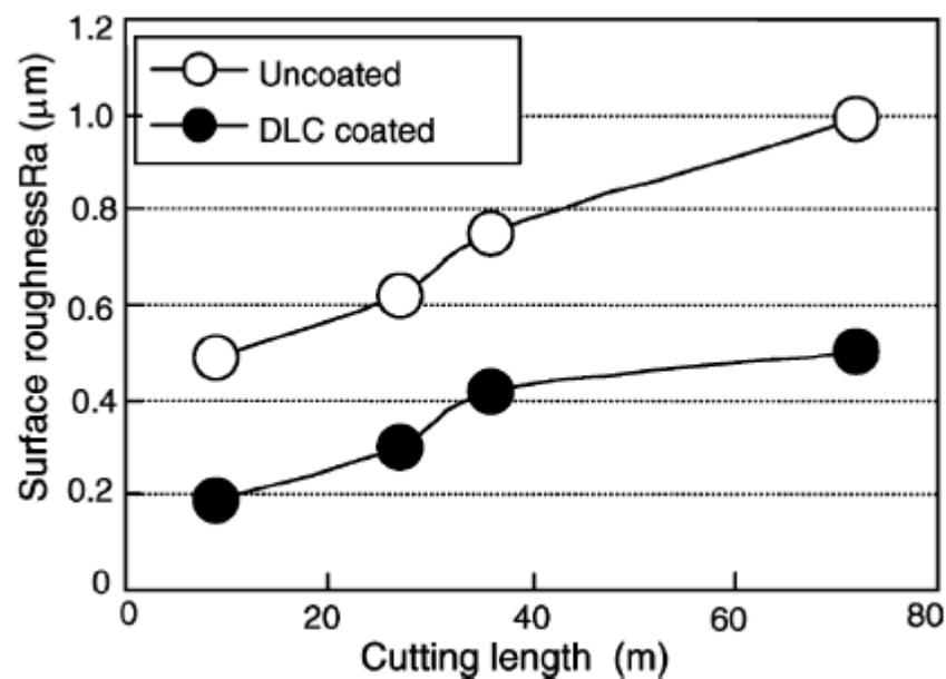
Figure 8. The variation of the surface roughness with along the cutting length [71].
