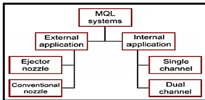
Figure 12. Minimum quantity lubrication delivery system categorizations [95].
