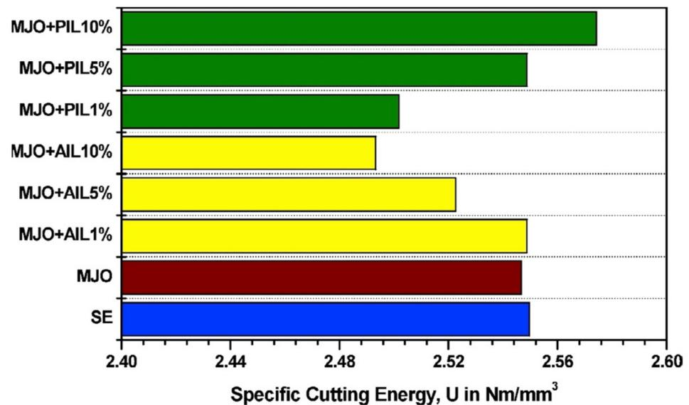
Figure 6. The variation of the specific cutting energy with respect to the mixture of modified jatropha oil (MJO) and AIL/PIL [66].
