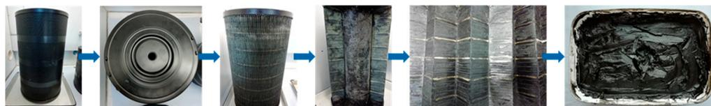
**Figure 4.** Flow sheet of dismantling, extraction of waste debris/sludge, example for SE\_01.
